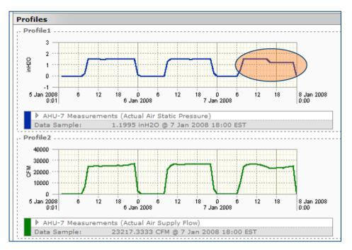
In this example, the slightly reduced static pressure setpoint had an annual savings of \$4,800 and 22-mTons of  $CO_2$  avoidance.
