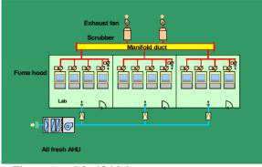
Figure 6 Manifold duct + VAV exhaust & supply system
