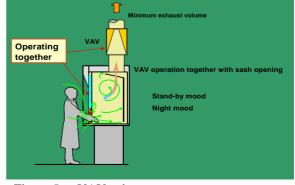
VAV exhaust system Figure 5 Operating with sash
