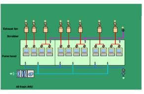
Figure 4 Conventional independent exhaust system
