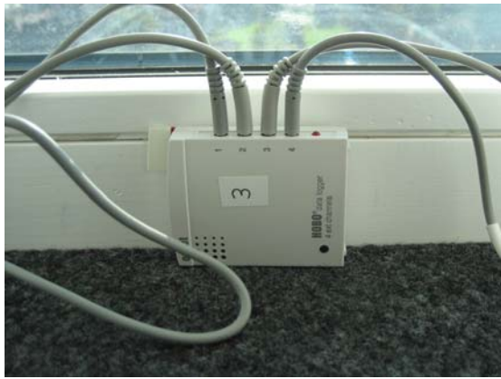
Figure 11a Temperature and humidity logger with four external channels
