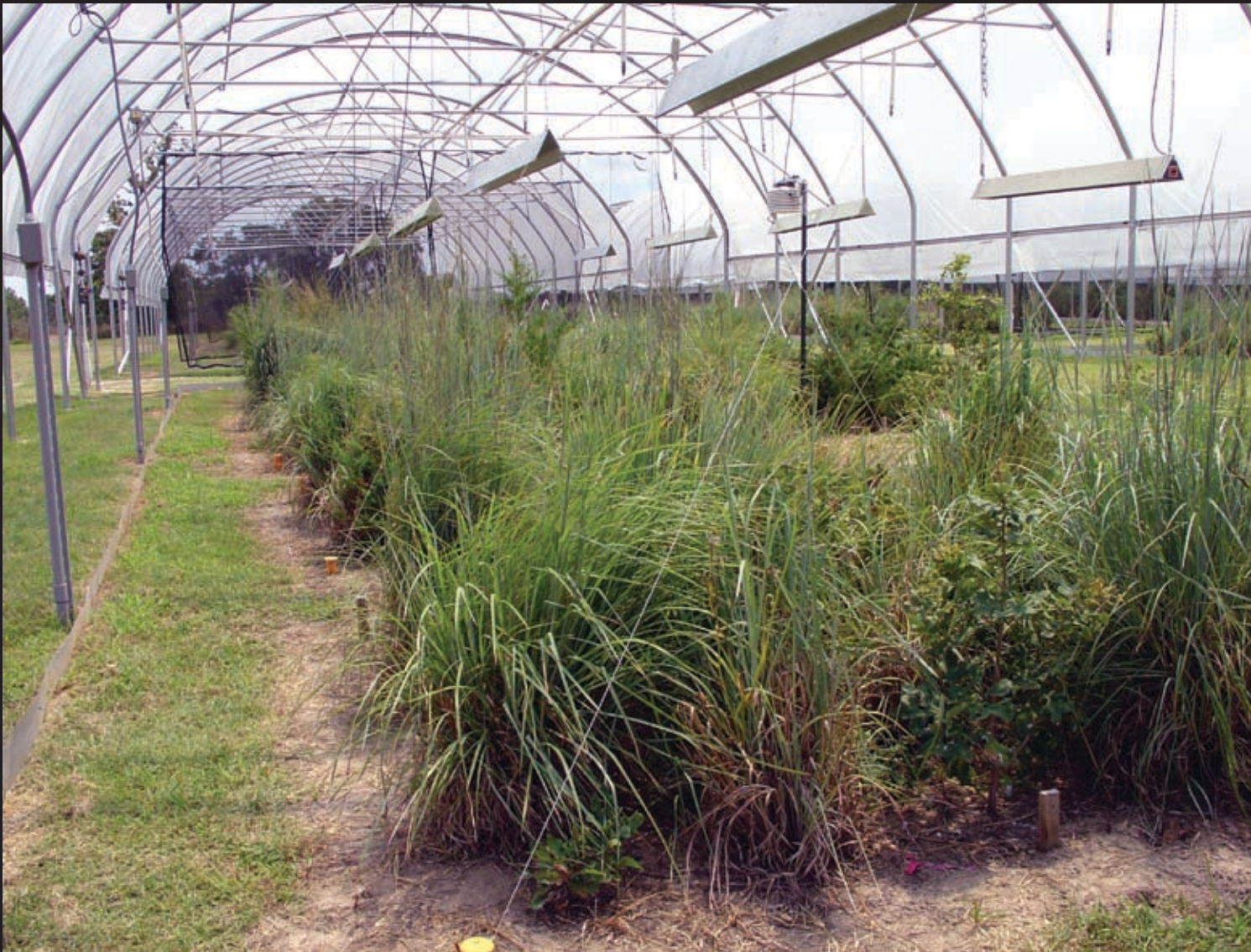
The Texas warming and rainfall manipulation experiment (WARM) is investigating the effects of climate change on oak savanna in Texas. Rainfall exclusion shelters and infrared lamps are used to control rainfall and simulate future climate warming. (Photo courtesy of MG Tjoelker.)
