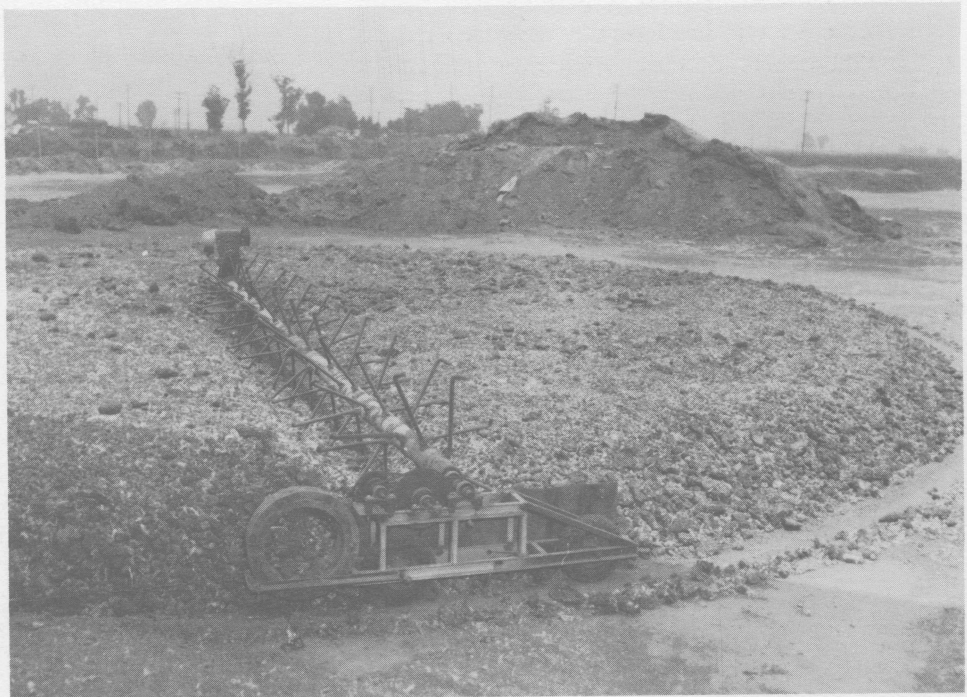
Figure 26. This mechanical "stirrer" is used to mix and dry droppings for sale as commercial fertilizer.
