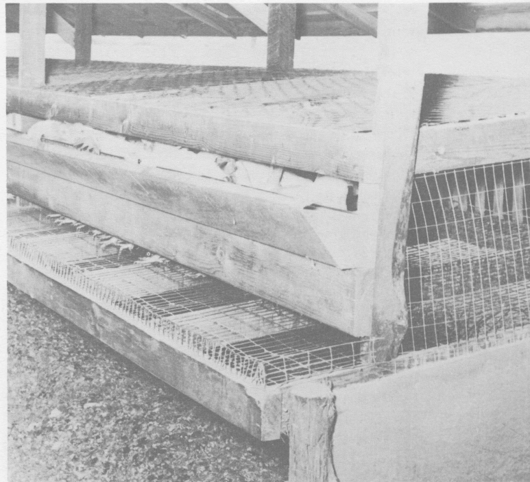
Figure 11. Moving the floor support from the area where the cage floor passes under the front wall to the edge of the "roll-out" tray will reduce the number of broken and dirty eggs.
