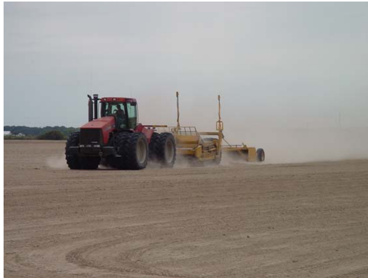
Figure 6. Land leveling is one of the best management practices cost-shared in the Arroyo Colorado watershed that levels the surface of the field to allow for uniform and efficient application of irrigation water and enhances conservation of soil and water resources.
