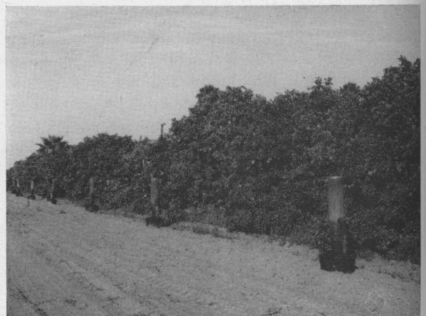
Fig. 14. The University return stack heater is a popular unit for grove heating since it burns with a clean flame and can be used at variable burning rates.
