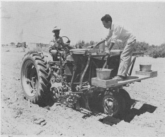
Figure 2. Tractor-mounted fertilizer apparatus used to apply various rates of nitrogen and phosphate to experimental test plots.
