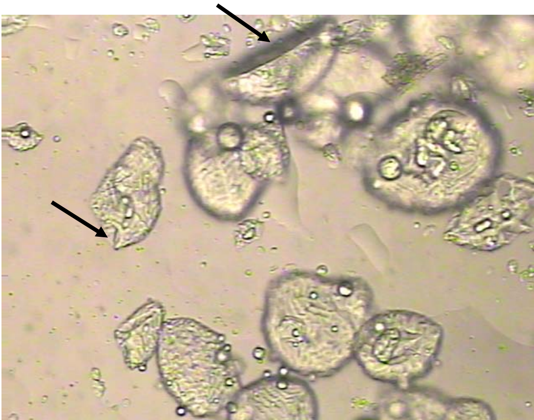
FIGURE 4. 10k 8 glyc 1 acryl PEGDA beads degradation example at one day after formation.
