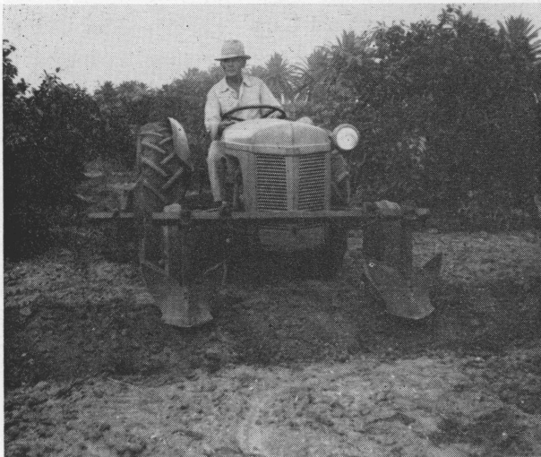
Figure 3. Middle breakers mounted on a front tool bar break the border (left) and facilitate passage of the tractor as the cross borders are being made (right).
