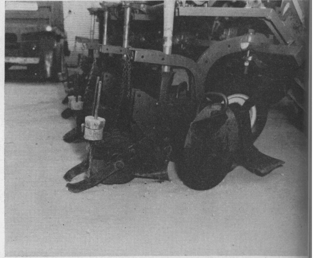
Figure 3. Plateau-profile planter consisted of modified lister bottom, disks on each side to cut furrows 2 to 3 inches deep and to leave a raised bed 10 inches wide at the top, narrow-shielded chisel seed-furrow opener, seed-firming wheel and short fishtail drags to cover seed.
