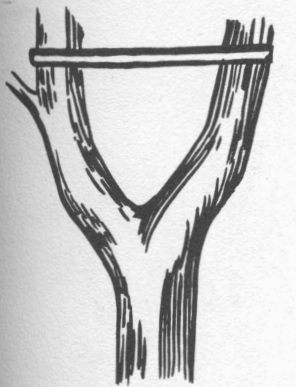
USE OF BAND OR WIRE FOR TREE BRACE
