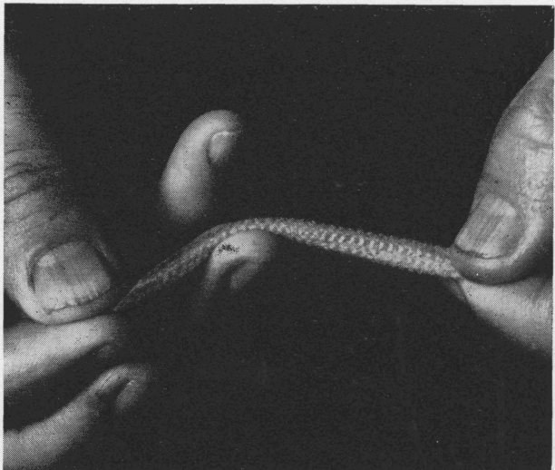
Testing wool for strength. If wool passes this test, it has sufficient strength.
