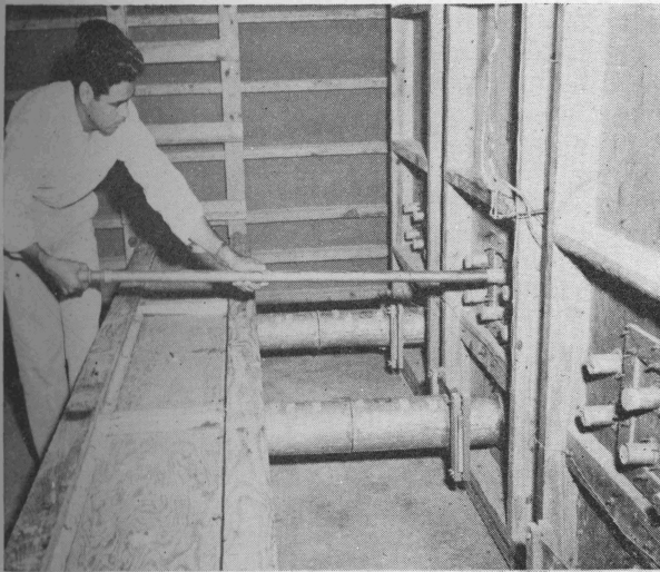
Figure 4. Samples of rice were drawn through ports in walls of small-scale bins (left). Cross-section of small-scale bin showing three levels at which samples were taken (right).
