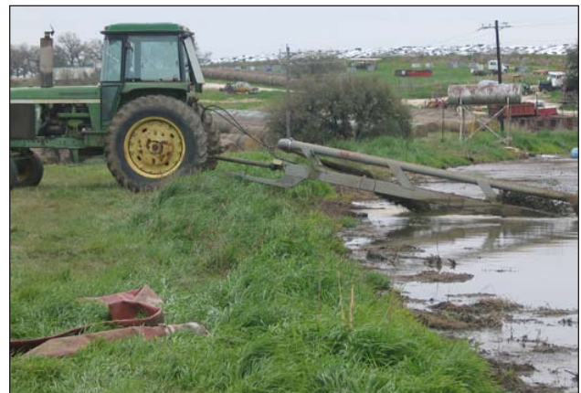
Figure 3: Chopper pump mixing the lagoon.
