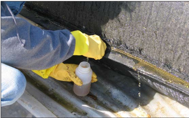
Figure 4: Sample collection from a Geotube®.
