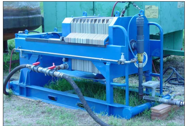
Figure 7: EC unit with iron electrodes built on a filter press frame.
