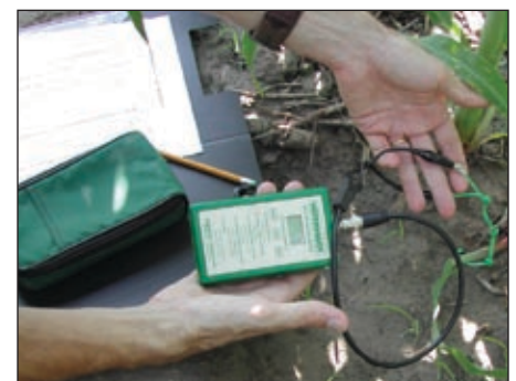
Figure 4. Using handheld meter for Watermark® sensor.
