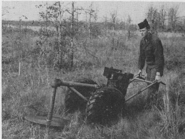
Figure 2. Motor-driven saws are effective in rapid clearing of small woodland or brush areas.
