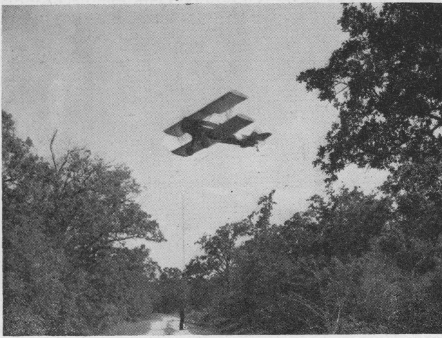
Figure 16. Fenuron pellets may be applied aerially in post and blackjack oak areas aerially during the spring growing season. Seeding and fertilizing equipment may be modified to release 16 pounds of pellets per acre.
