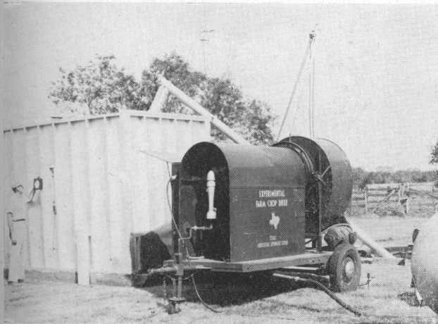
Figure 28. This portable batch dryer, used in the studies, consisted of a drying bin 7 by 14 feet with walls 6 feet high. A perforated steel floor separated the drying bin from the air chamber. Grain was loaded to the desired depth on the drying floor and heated air was forced into the air chamber and through the grain until the moisture content was reduced to a safe limit. The experimental farm crop dryer attached to the batch drying bin utilized LP gas and electric power during operation.
