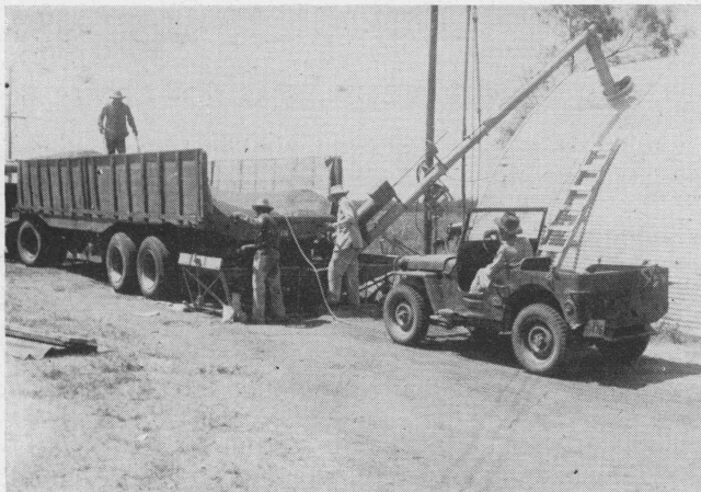
Figure 15. An auger loader and grain tow board were used for handling grain in and out of storage.
