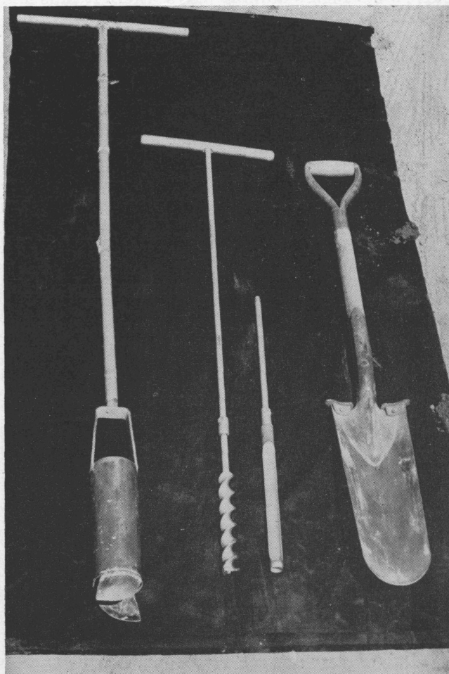
Figure 10. Some equipment for obtaining soil samples to estimate available moisture includes an orchard auger, soil auger with soil tube attachment and a sharpshooter.
