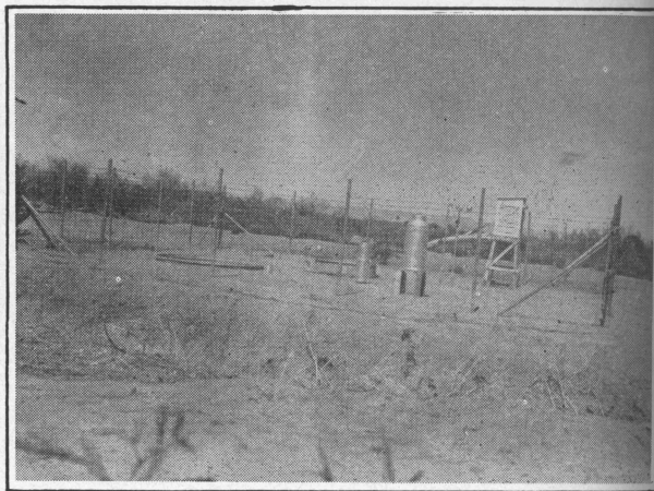
Figure 11. Installation of anemometers for recording wind movement at various elevations above ground surface and stressing the importance of recognized standard installation.
