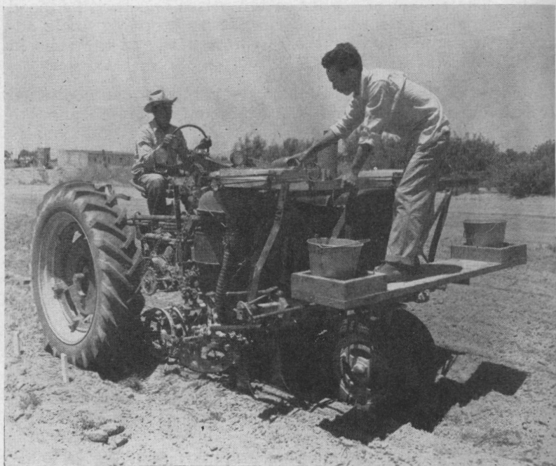
Figure 1. Experimental plot fertilizer distributor mounted on tractor.
