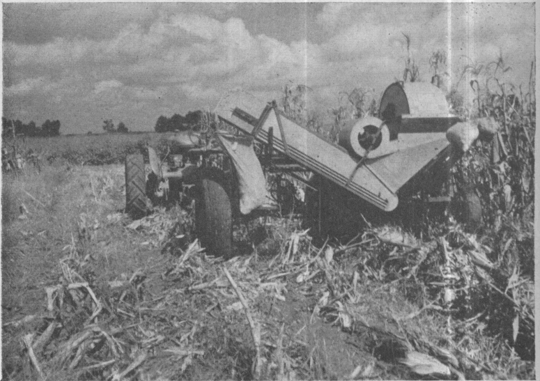
Figure 7. Close-up view of corn picker showing sacking attachment with sack partially filled with corn. Note that a counter-balance weight was necessary to balance the machine over the wheels when the elevator extension was removed.
