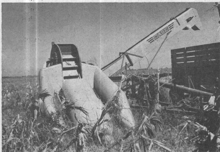
Figure 3. Showing corn picker with long extension wagon elevator in position to convey the harvested corn from the picker to the wagon.
