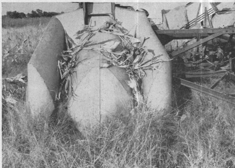
Figure 11. Showing how stalks of Surcropper broke off and collected on the machine when harvest was delayed until October.
