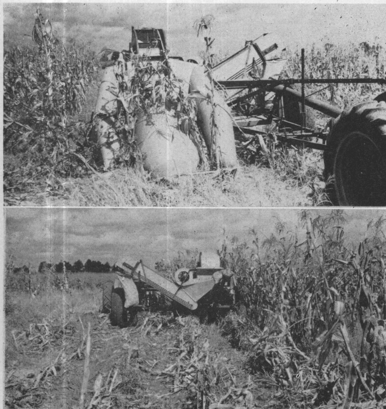
Figure 6. Showing front and rear views of corn picker in operation and equipped with sacking attachment.
