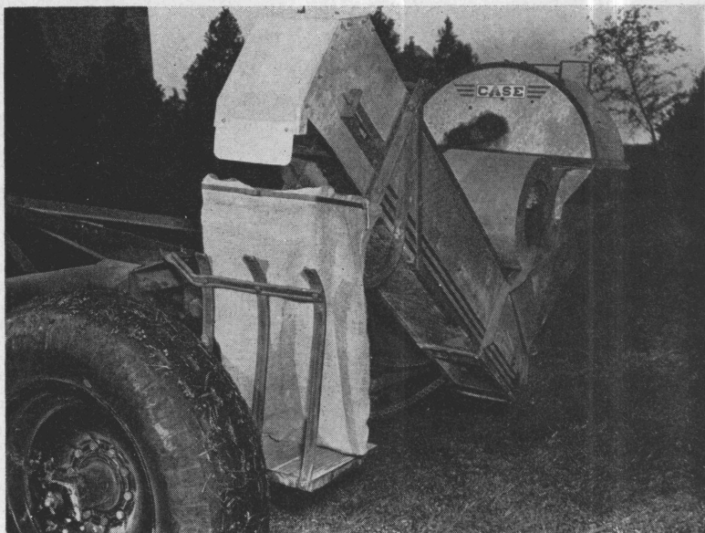
Figure 5. Special sacking attachment substituted for extension wagon elevator so that corn could be sacked as harvested. The sack of corn is supported by a small platform.
