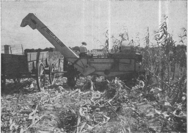
Figure 18. Rear view of corn picker equipped with husking attachment.
