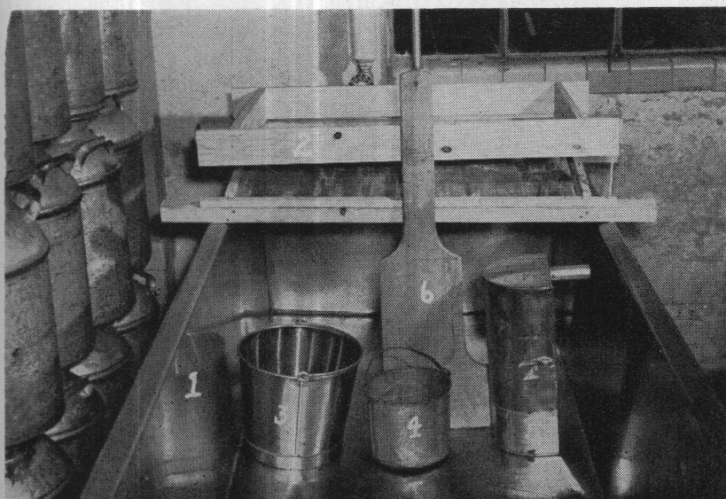
Fig. 2. The Manufacturing Equipment Used. 1. Cheese vat, 2. Drain rack, 3. Pail, 4. Curd Pail, 5. Vat strainer, 6. Paddles.
