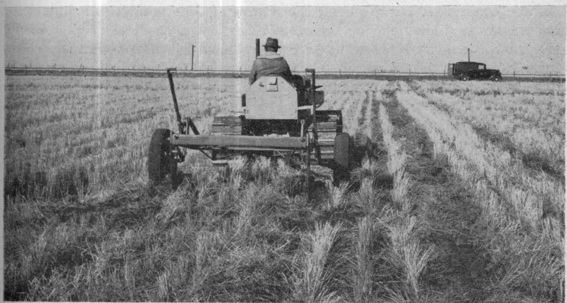
Fig. 11. One method of stubble land plowing designed to leave the trash on the surface.
