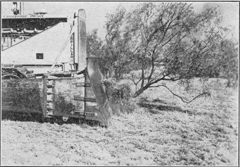
Fig. 24. Machine designed for uprooting mesquite and other brush on range land. It is necessary to remove most of the root system of mesquite for the reason that this plant sprouts readily from the roots.
