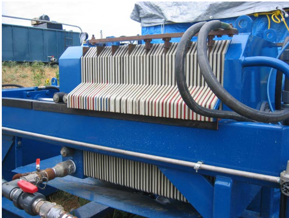
Fig. 6. The EC Unit with Iron Electrodes, Built on a Filter Press Frame
