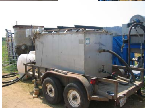
Fig. 5. The Dissolved Air Flotation (DAF) Unit
