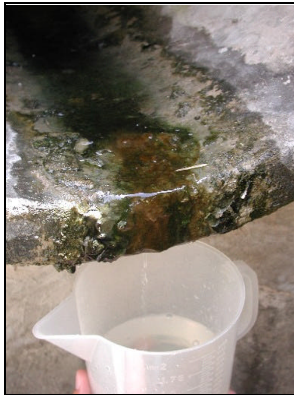
Figure 8. Close up of the graduated beaker used to measure gate leakage.
