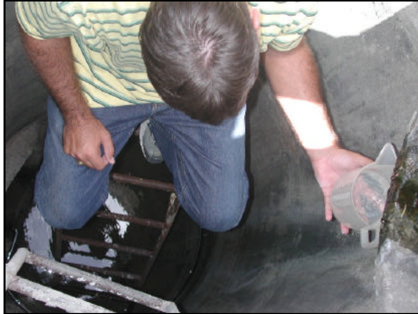
Figure 7. Measuring the leakage rate through a turnout gate inside a standpipe.
