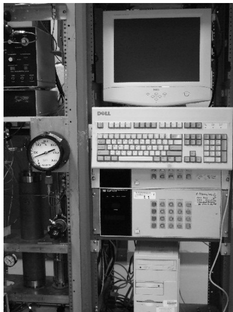
Fig. 3.5- Data recording system consists of a data logger and a personal computer.
