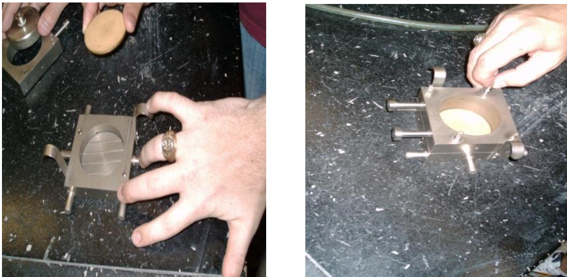
Fig. 5.4. Direct shear box assembly (Biscontin 2006)
