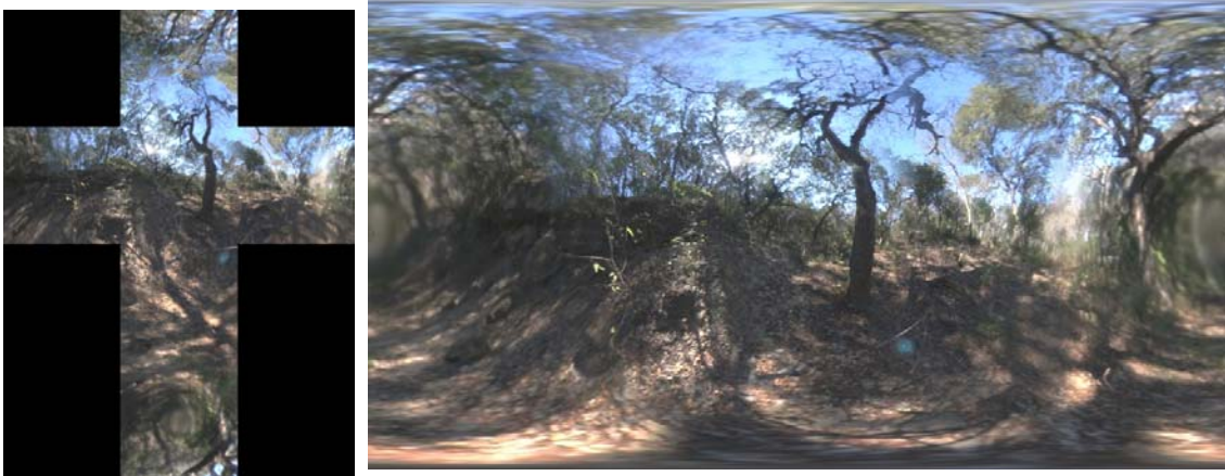
Figure 6. Cubic (left) and spherical (right) environment map projections
