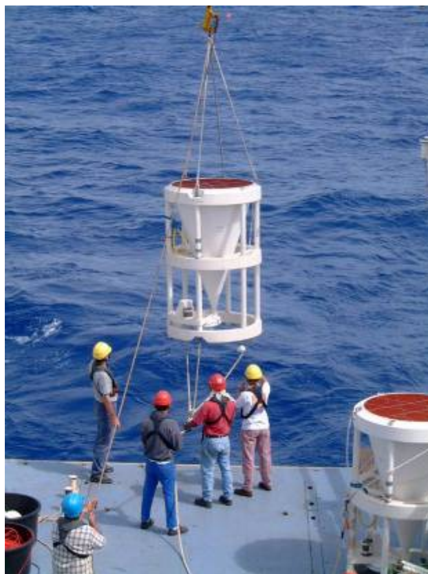
Figure 3: Floating sediment trap deployment during the BIOSOPE cruise in the Southeastern Pacific.
