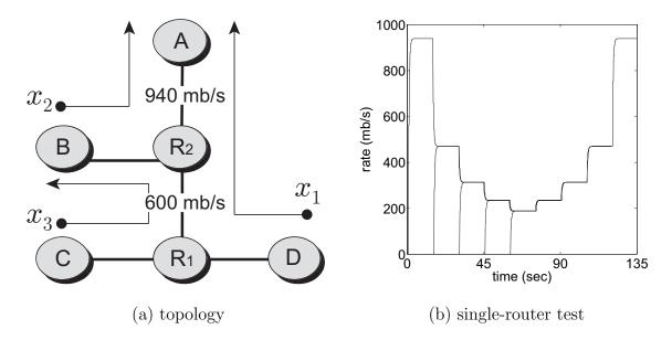
Fig. 43. Single-router Linux experiments with JetMax ( $\tau = 0.6$ ).
