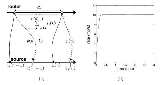
Fig. 20. Proper EMKC implementation: (a) graphical explanation of the algorithm;
