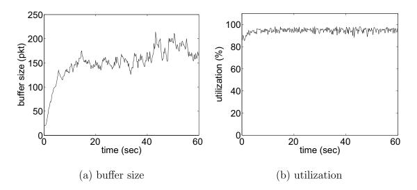
Fig. 49. ABS in a single link of capacity 10 mb/s shared by 20 FTP and 100000 HTTP flows ( $u^* = 95\%$  and  $p^* = 1\%$ ).
