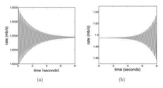
Fig. 8. (a) Behavior of TFRC for different stationary points: (a)  $r^* = 1.503C$ ; (b)  $r^* = 1.494C$ .
