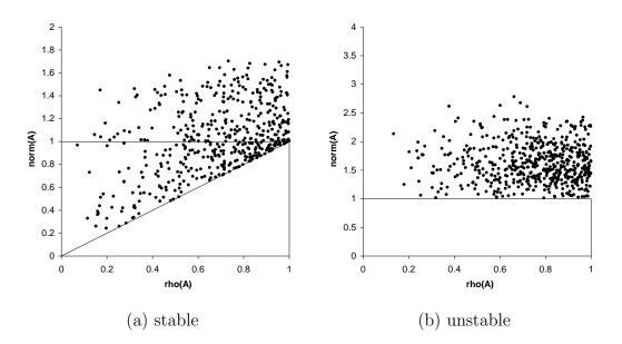
Fig. 12. Delayed stability as a function of  $\rho(A)$  and  $||A||_2$ .
