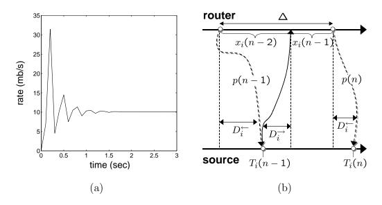
Fig. 19. Naive EMKC implementation: (a) one ns2 flow ( $\alpha = 100$  kb/s,  $\beta = 0.9$ , and  $\Delta = 50$  ms) passes through a bottleneck link of capacity 10 mb/s; (b) inconsistent feedback and reference rate.
