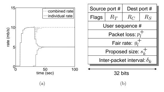
Fig. 35. (a) JetMax ( $\tau = 0.6$  and  $\gamma = 1$ ) with proposed rate in  $\mathcal{T}_1$ ; (b) format of the JetMax packet header.
