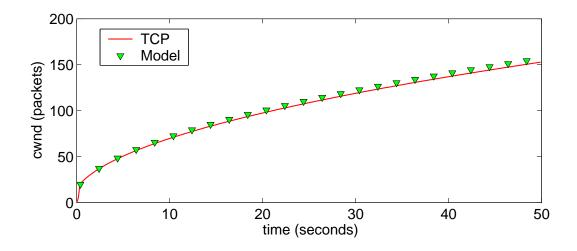
Fig. 5. The congestion window of a single TCP flows under delay.
