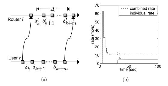
Fig. 33. (a) The relationship between control interval Δ<sub>l</sub> and inter-packet interval δ<sub>k</sub>;
