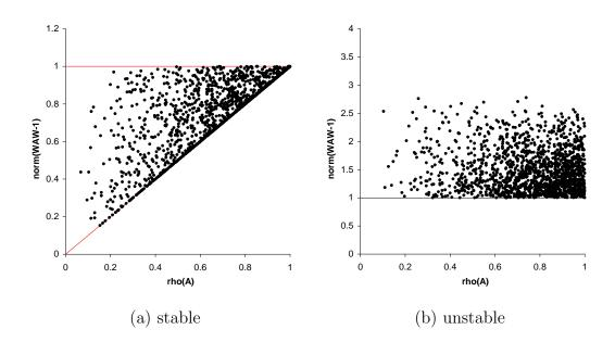
Fig. 13. Delayed stability as a function of  $\rho(A)$  and  $\inf_{W} ||WAW^{-1}||_2$ .
