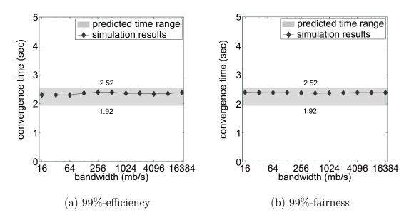
Fig. 41. Convergence time of JetMax ( $\tau = 0.6$  and  $\gamma = 1$ ) as a function of bottleneck capacity C in ns2.
