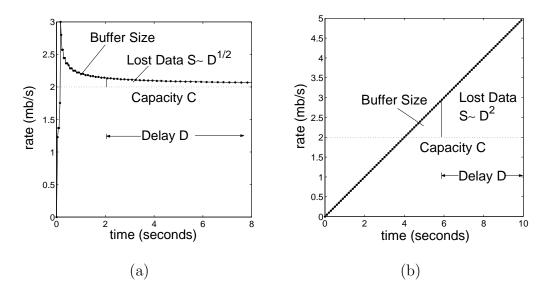
Fig. 6. (a) Rate adjustment of window-based protocols under delays. (b) Rate adjustment of rate-based protocols under delays.
