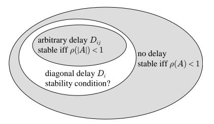
Fig. 10. Illustration of the current research status of delay-independent stability of system (31) under different types of delays.
