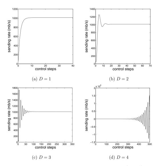
Fig. 14. Stability of Kelly control under different feedback delays ( $\kappa = 1/2, \omega = 10$  mb/s, and C = 1,000 mb/s).
