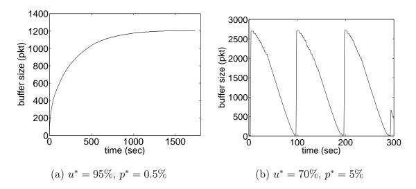
Fig. 46. ABS  $(I_u = I_p = 3000 \text{ and } T = 200 \text{ ms})$  without parameter training in a network with a single link of capacity 10 mb/s and 20 TCP flows.
