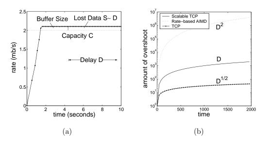
Fig. 7. (a) Rate adjustment of Scalable TCP under delay. (b) Comparison of lost data per overshoot in TCP, Scalable TCP, and rate-based AIMD.
