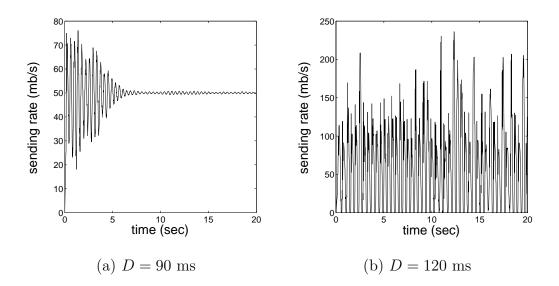
Fig. 15. Simulation results of the classic Kelly control under different delays ( $\kappa = 1/2$ ,  $\omega = 20$  kb/s, C = 50 mb/s).
