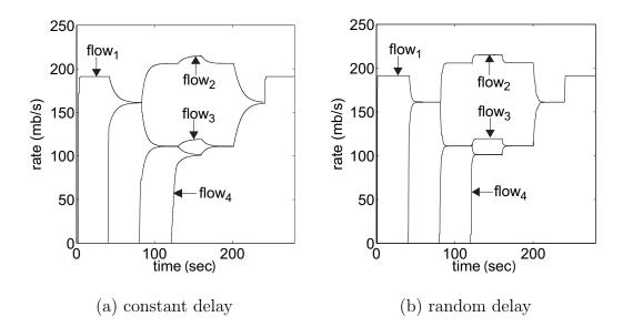
Fig. 23. Proper implementation of EMKC ( $\alpha = 10 \text{ mb/s}$ ,  $\beta = 0.9$ , and  $\delta = 0.01$ ) in the "parking lot" topology.
