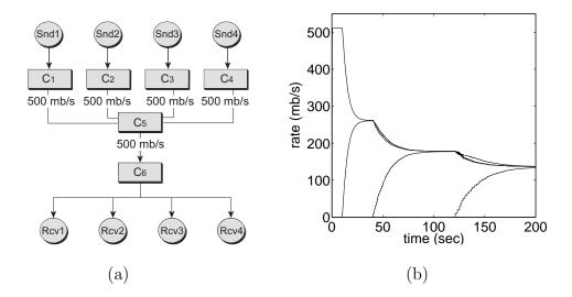
Fig. 21. Four EMKC ( $\alpha = 10 \text{ mb/s}$ ,  $\beta = 0.9$ , and  $\Delta = 100 \text{ ms}$ ) flows in the "dumb bell" topology.
