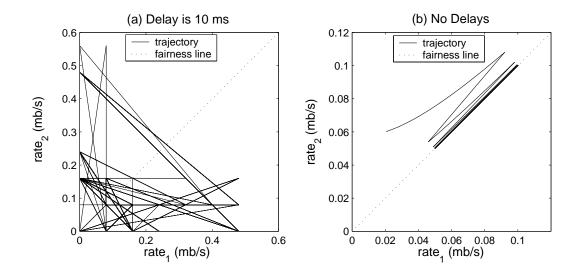
Fig. 4. Trajectories of two TCP flows: (a) 10 ms delay; (b) Instantaneous feedback.
