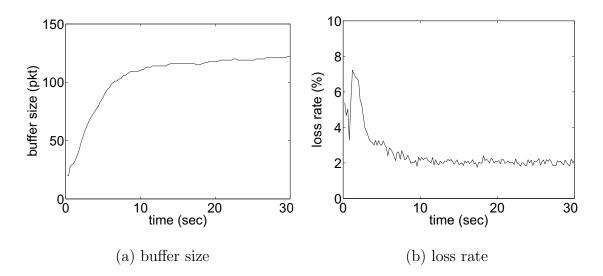
Fig. 50. ABS in a single link of capacity 10 mb/s shared by 20 FTP, 20 HTTP, and 20 UDP flows ( $u^* = 90\%$  and  $p^* = 2\%$ ).
