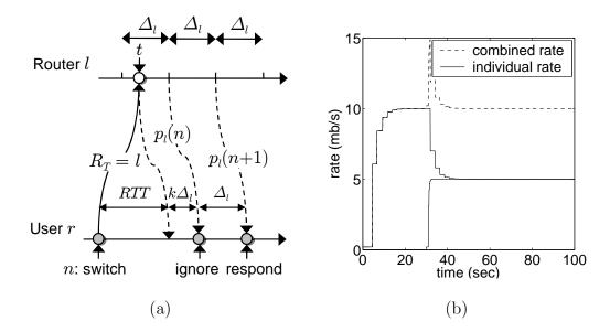
Fig. 34. (a) The scenario where the bottleneck switching occurs in the middle of the router's control interval; (b) JetMax ( $\tau = 0.6$  and  $\gamma = 1$ ) with the proper bottleneck switching scheme in  $\mathcal{T}_1$ .
