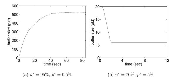
Fig. 47. ABS with parameter training in a network with a single link of capacity 10 mb/s and 20 TCP flows.
