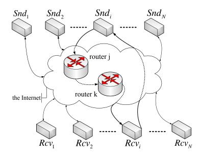
Fig. 9. Model of the network and directional feedback delays.
