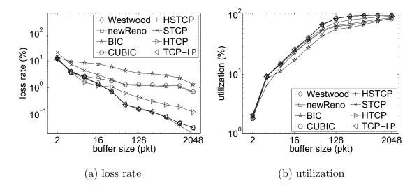
Fig. 45. Effect of buffer size b on loss rate p and utilization u of several TCP variants. and u are monotonic functions of b. Note that the loss curves of CUBIC and STCP in Figure 45(a) appear to be flat when b is between 64 and 1024 packets; however, we verified numerically that they are actually monotonically decreasing.
