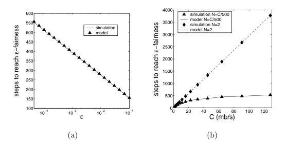
Fig. 16. (a) Verification of model (108) against EMKC simulations (C = 1 mb/s,  $\alpha = 10$  kb/s, and  $\beta = 0.5$ ). (b) Exponential and linear rates of convergence to fairness for EMKC ( $\varepsilon = 0.1$ ).
