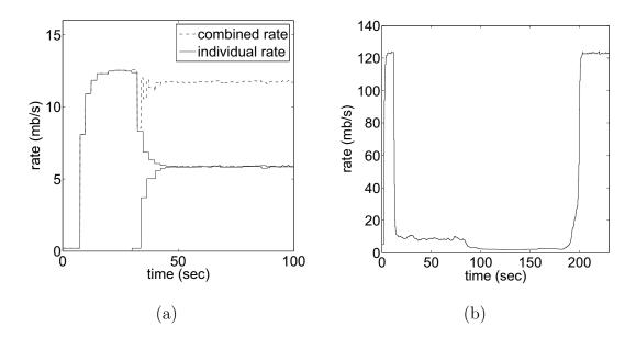
Fig. 39. JetMax ( $\tau = 0.6$  and  $\gamma = 1$ ) under random packet loss: (a)  $\mathcal{T}_1$  with 10% forward-path loss; (b) "parking lot" topology with mice flows and random loss.
