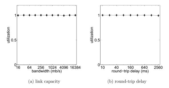
Fig. 40. Utilization of the bottleneck in JetMax ( $\tau = 0.6$  and  $\gamma = 1$ ) under different link capacities and round-trip delays in ns2.
