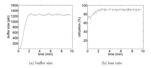
Fig. 51. ABS in a single link of capacity 100 mb/s shared by 10 Reno, 10 HSTCP, 10 STCP, 10 HTCP, and 10 Westwood flows ( $u^* = 90\%$  and  $p^* = 2\%$ ).
