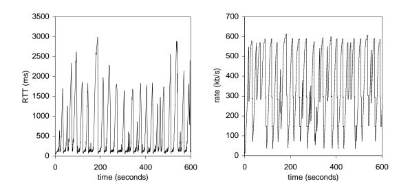
Fig. 2. Video streaming over 512-kb/s residential DSL. Evolution of the RTT (left) and that of the IP-layer sending rate (right).
