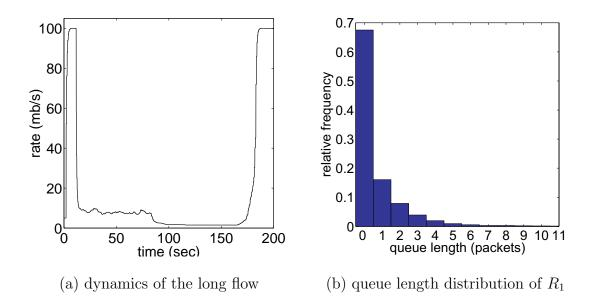
Fig. 38. Multi-link performance of a long JetMax flow ( $\tau = 0.6$  and  $\gamma = 1$ ) in the presence of mice traffic.
