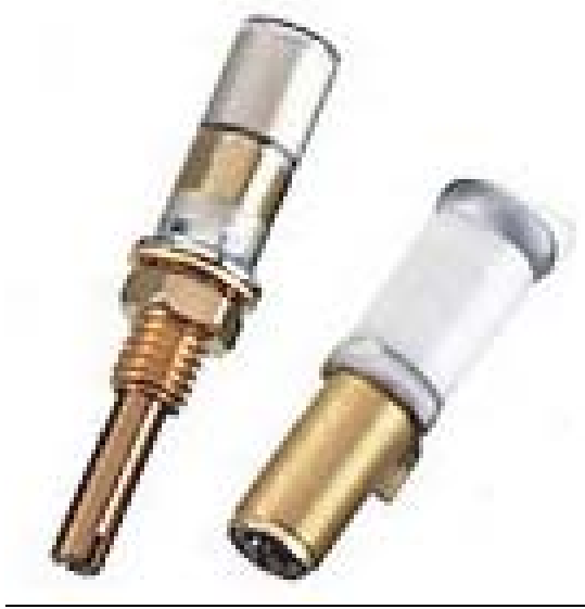
Figure 27 The cap on the right is currently used on the coil. A tuning stick with a small screw driver has to be mounted on this capacitor. The diameter of this screw is 0.3cm. The mechanical stability of this tuning stick on a small surface area (0.3cm) is an area of concern. Thus, we should use the capacitor on the left with a shaft on the capacitor. The advantage of the shaft is that it does not need a small screw driver at the end of the tuning stick. The tuning stick can be glued to the large surface area of the shaft.
