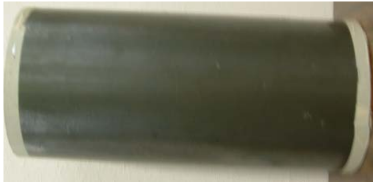
Figure 6(a) Dupont pyralax shield wrapped on the acrylic former.
