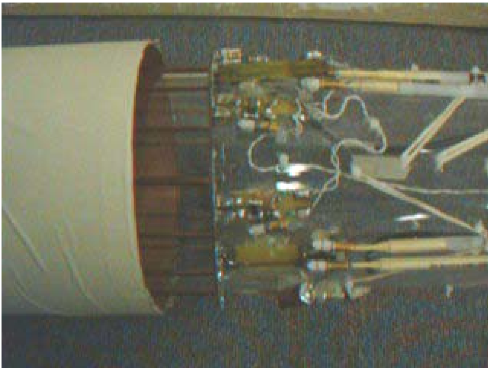
Figure 15 The quadrature drive implemented on the shielded birdcage coil. The coil was fed through a balun and matching/tuning circuit. There were 4 tuning sticks interfacing the match/tune circuit. The twisted pair of wires supply the DC to the diodes required for detuning the coil.
