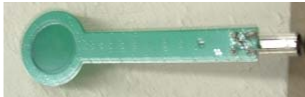
Figure 23 Probe used for the homogeneity measurements for all 3 coils. This probe was commercially obtained.
