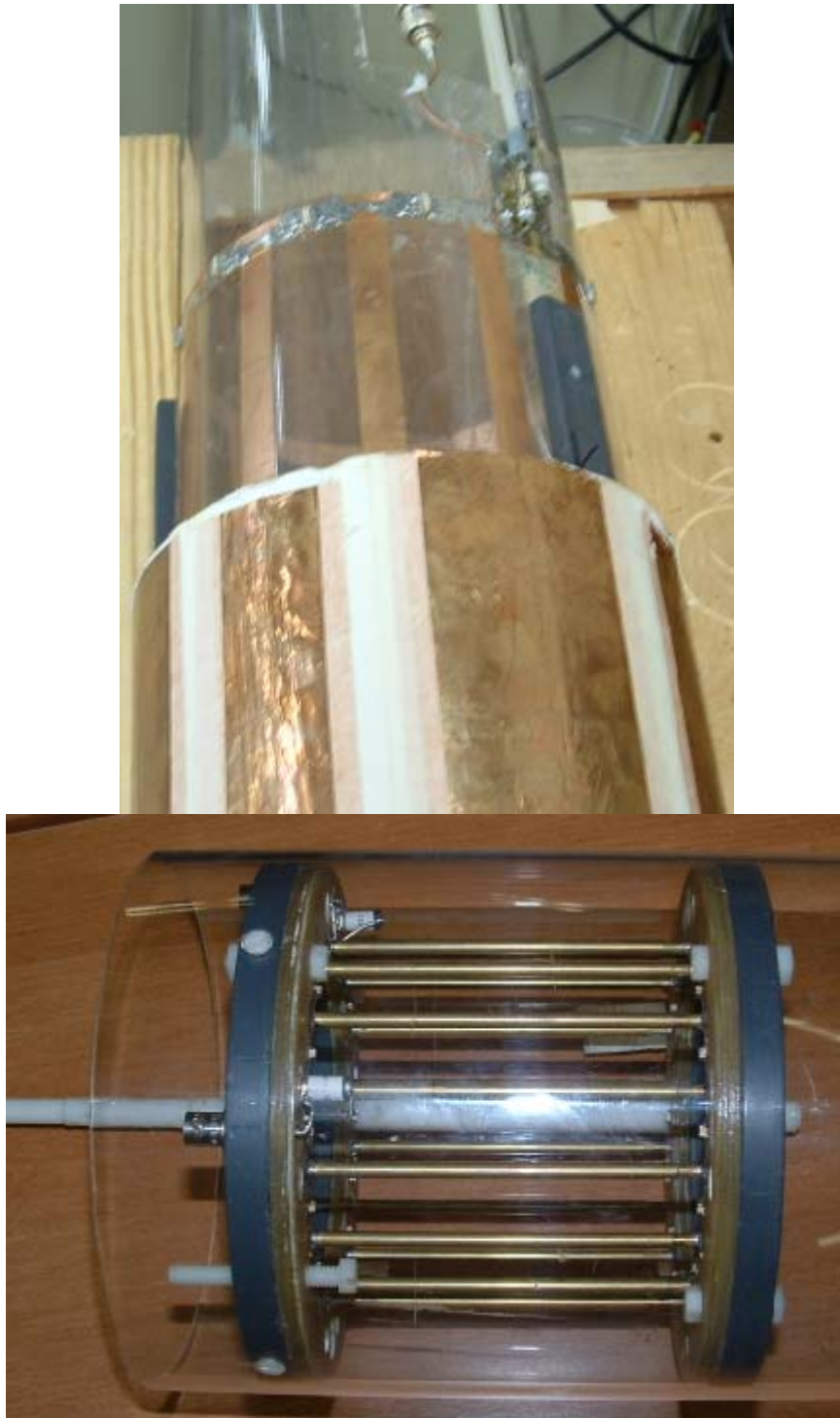
Figure 20 Top is a picture of the “Cu tape-15.5cm” coil and bottom is the “trombone-10cm” unshielded coil. The coil length is 25cm, coil diameter is 15.5cm, shield diameter is 17.2cm of the former coil and coil length is 15cm and coil diameter is 10cm of the “trombone-10cm” coil.
