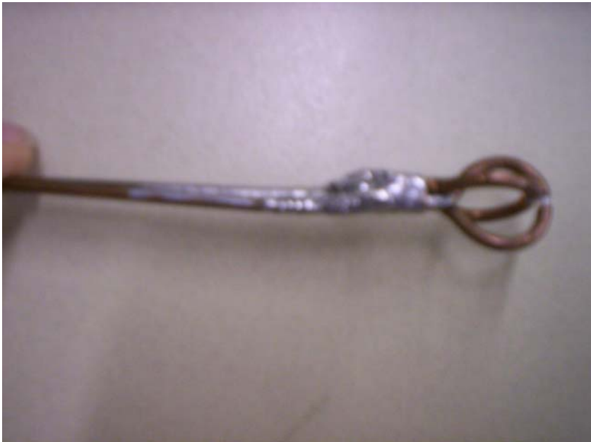
Figure 1 Crossed-probe used to measure the two orthogonal resonant modes. A description of the voltage detected by this probe is given in this section.
