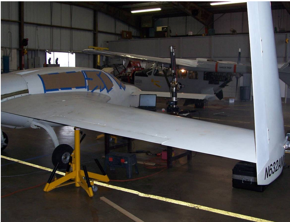
Figure A.5 Velocity XL-5 RG on Aircraft Jacks during Surface Measurements
