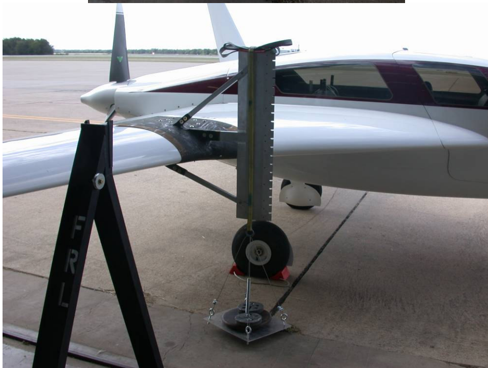
Figure A.102 Hanging 20 kg (45 lbs) From the Pressure Rake to Simulate a 2-G Pull-up
