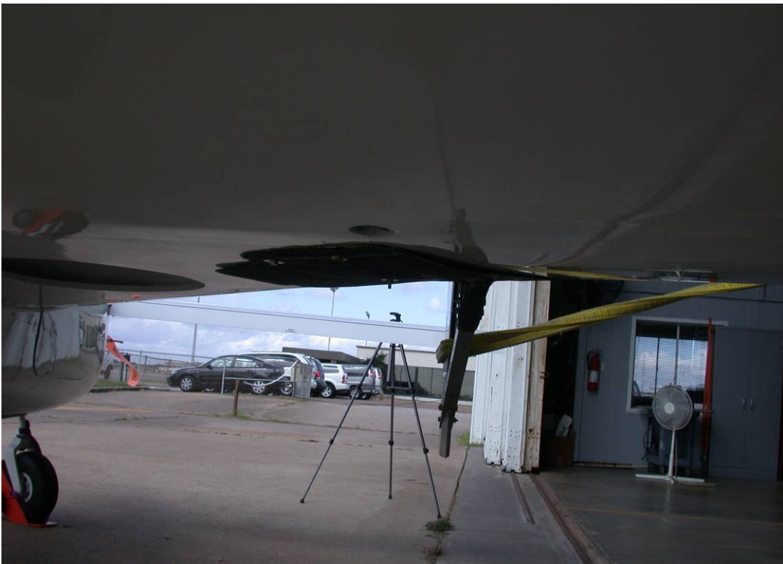
Figure A.101 Monitoring for Deflections or Yielding in the Pressure Rake during Static Load Test
