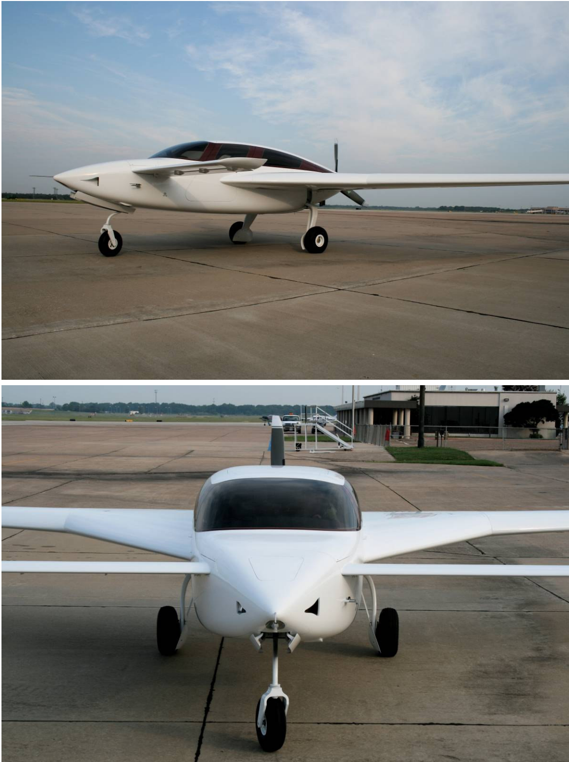
Figure A.90 24-inch 5-hole Probe Extending out the Nose of the Velocity
