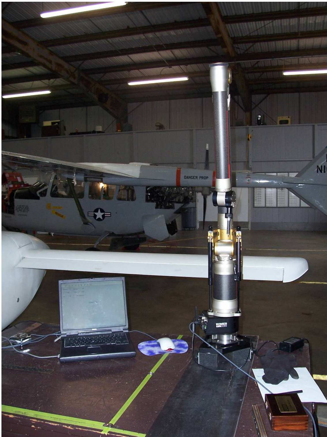
Figure A.6 CMM Configuration during Measurements with Stand, Coordinate System Origin, and Acquisition Program
