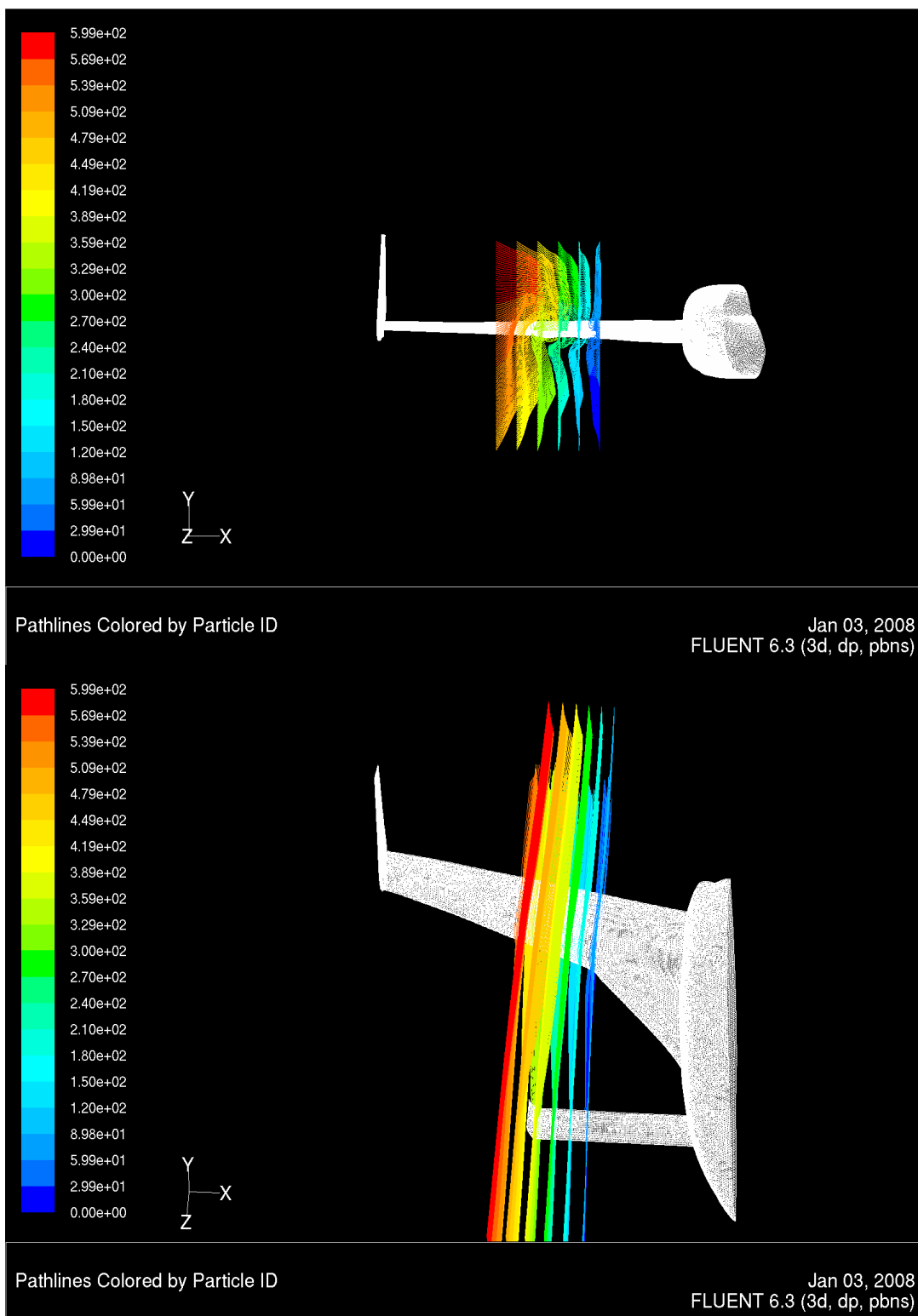
Figure A.67 Pathlines Exploring the Spanwise Range of Influence of the Tip Vortex at 0^\circ AoA, 100 m/s
