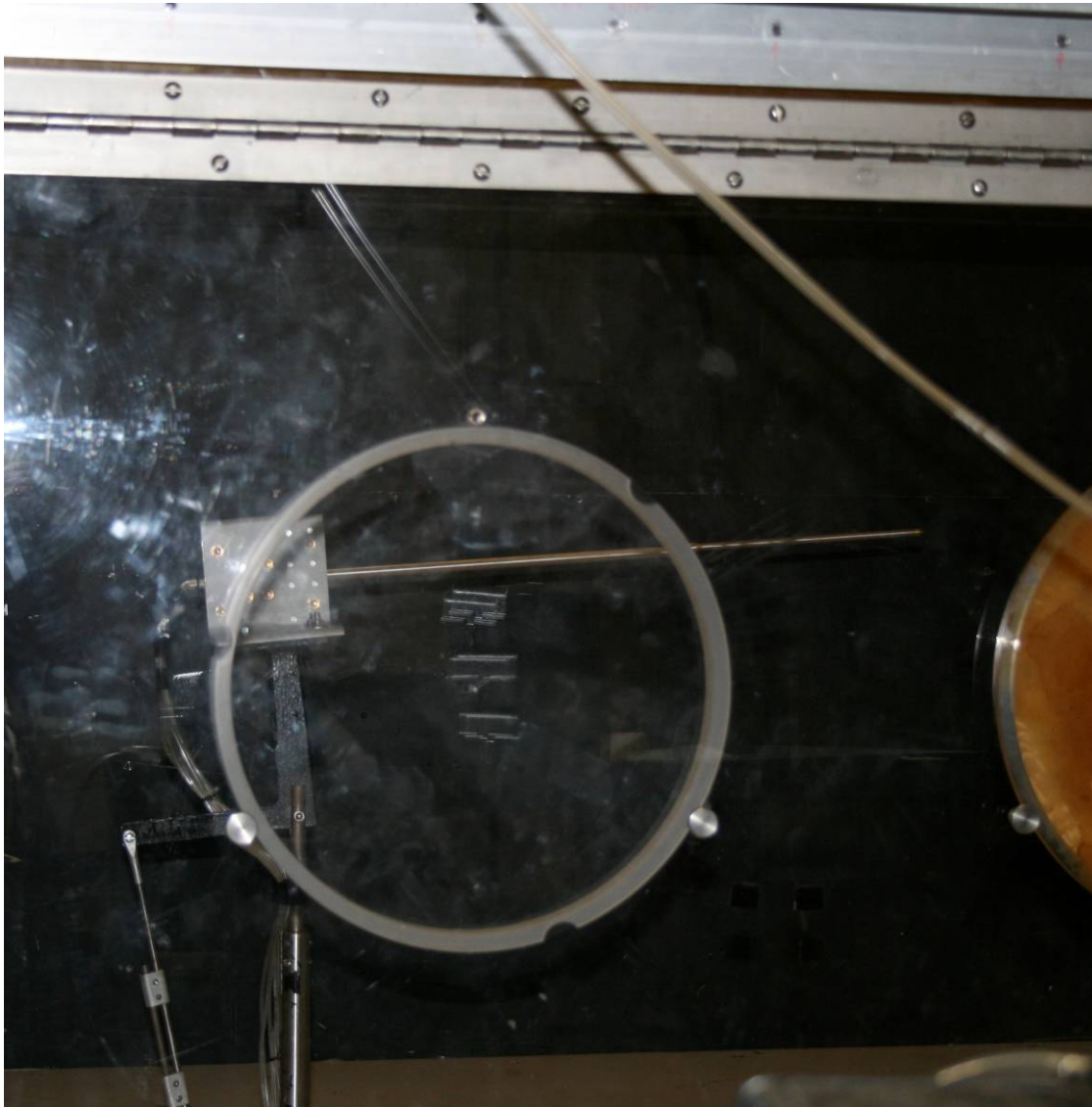
Figure A.85 24-inch 5-hole Probe Mounted in the 3'x4' ELD Wind Tunnel
