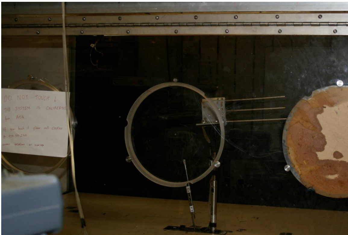
Figure A.86 12-inch 5-hole Probe Mounted in the 3'x4' ELD Wind Tunnel Isolated and with the Pitot Probes on Either Side at the Spacing Used in the Pressure Rake
