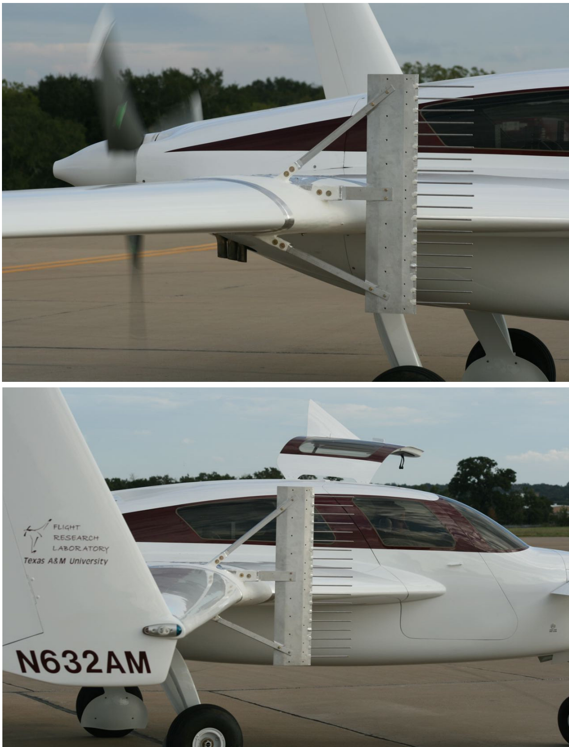
Figure A.104 Engine Run-up Test with the Pressure Rake
