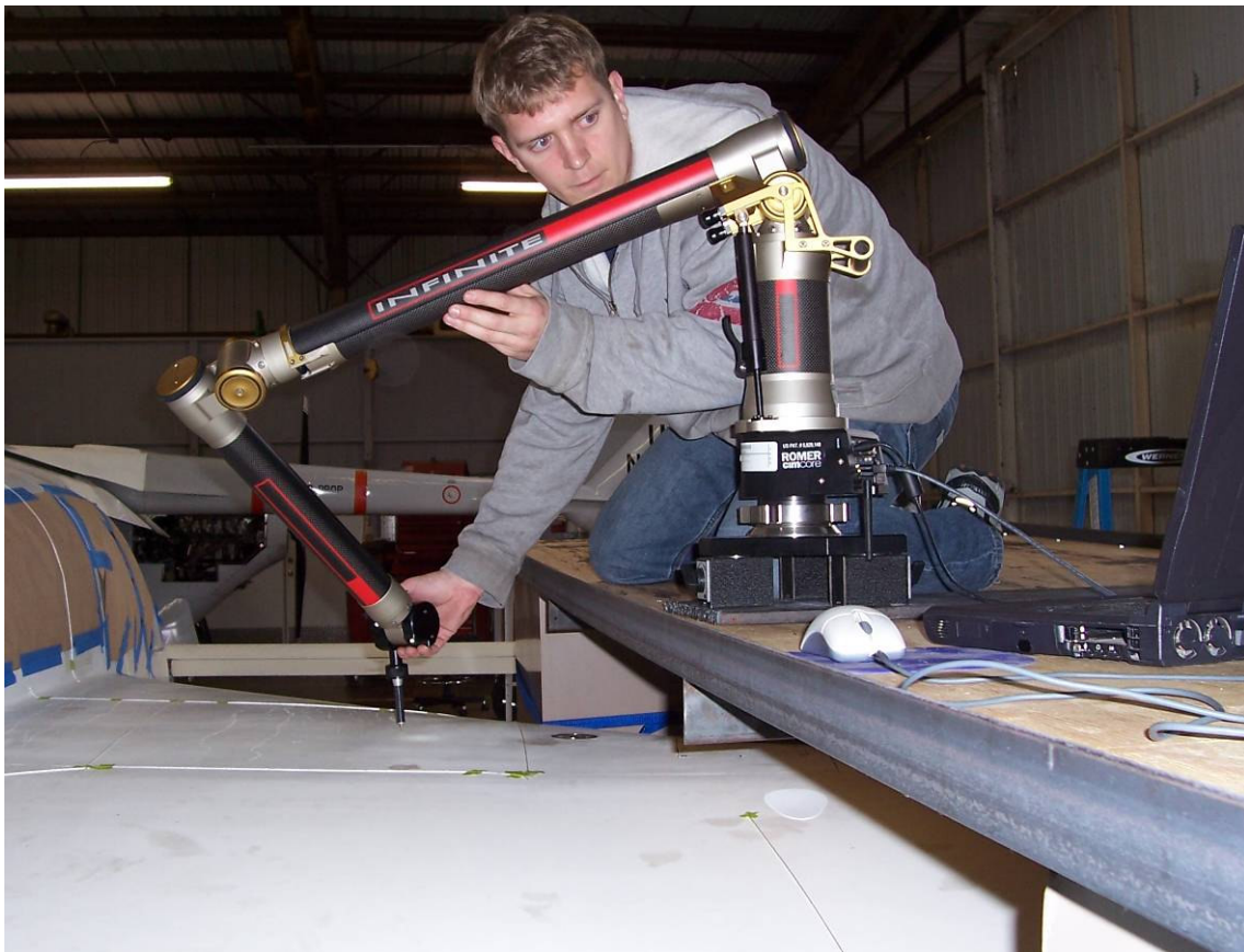
Figure A.9 Using the CMM on the Scaffolding above the Aircraft
