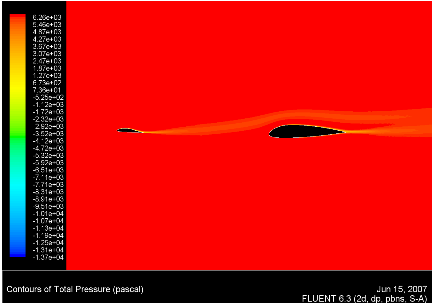
Figure A.49 Gauge Total Pressure Plot of the Velocity Canard and Wing Using the Spalart-Allmaras Turbulence Model at 5° AoA, 100 m/s
