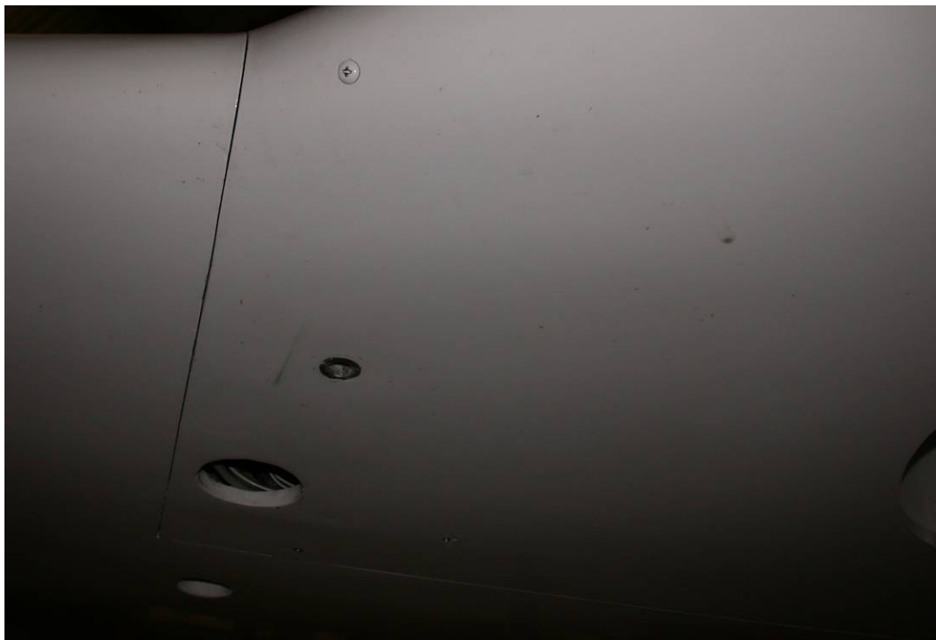
Figure A.72 Available Attachment Points at the Crank Location on the Upper and Lower Surface of the Wing of the Velocity
