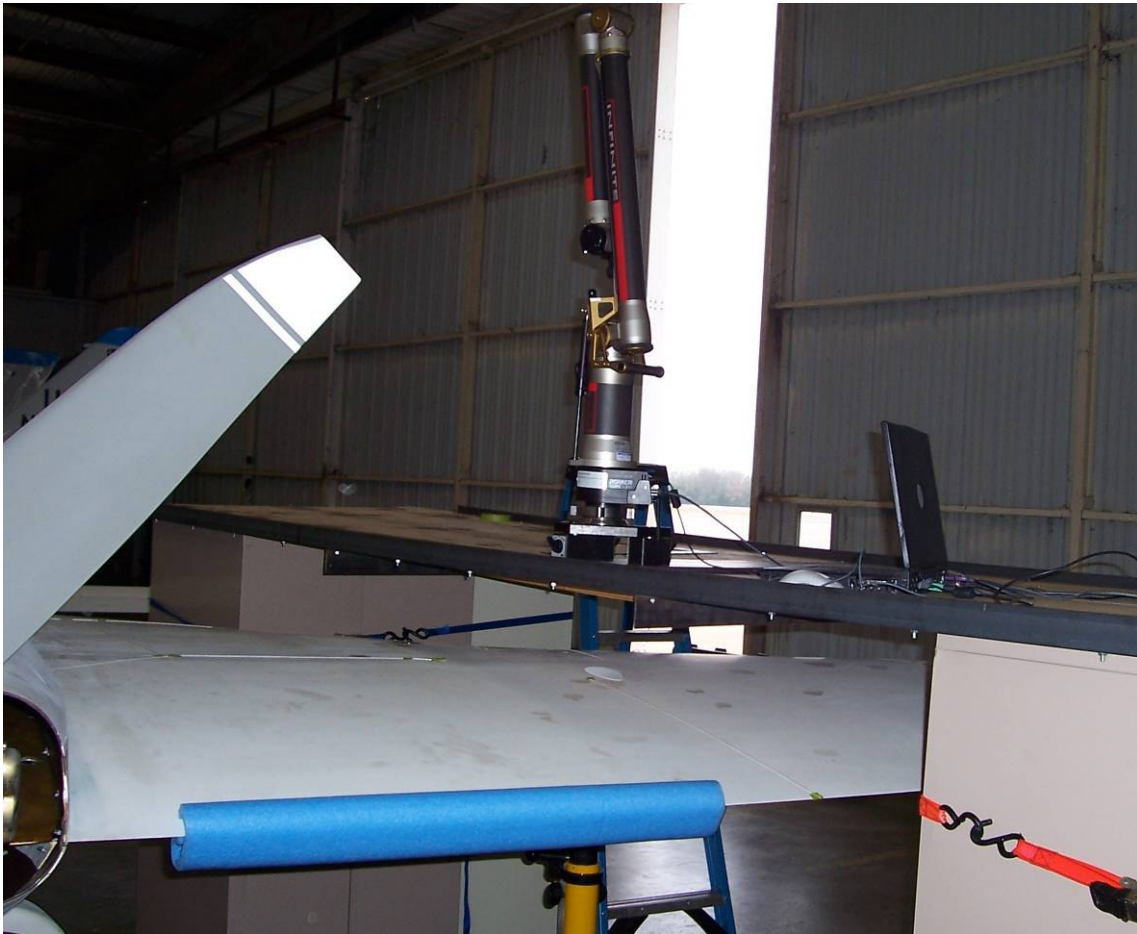
Figure A.8 CMM on Scaffolding over the Top of the Aircraft Wing
