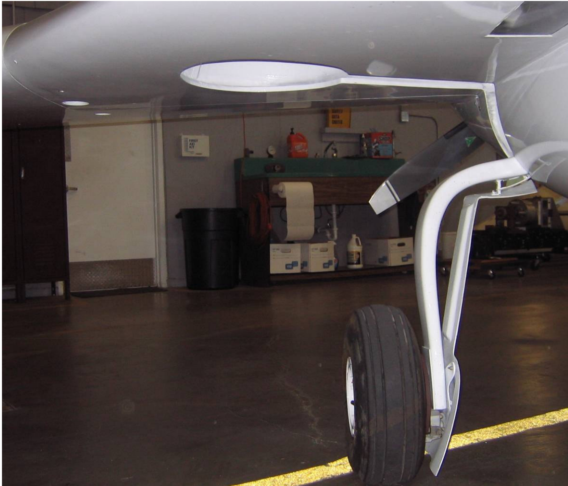
Figure A.13 Picture of the Main Gear of the Velocity with Gear Well and Wheel Cover Visible
