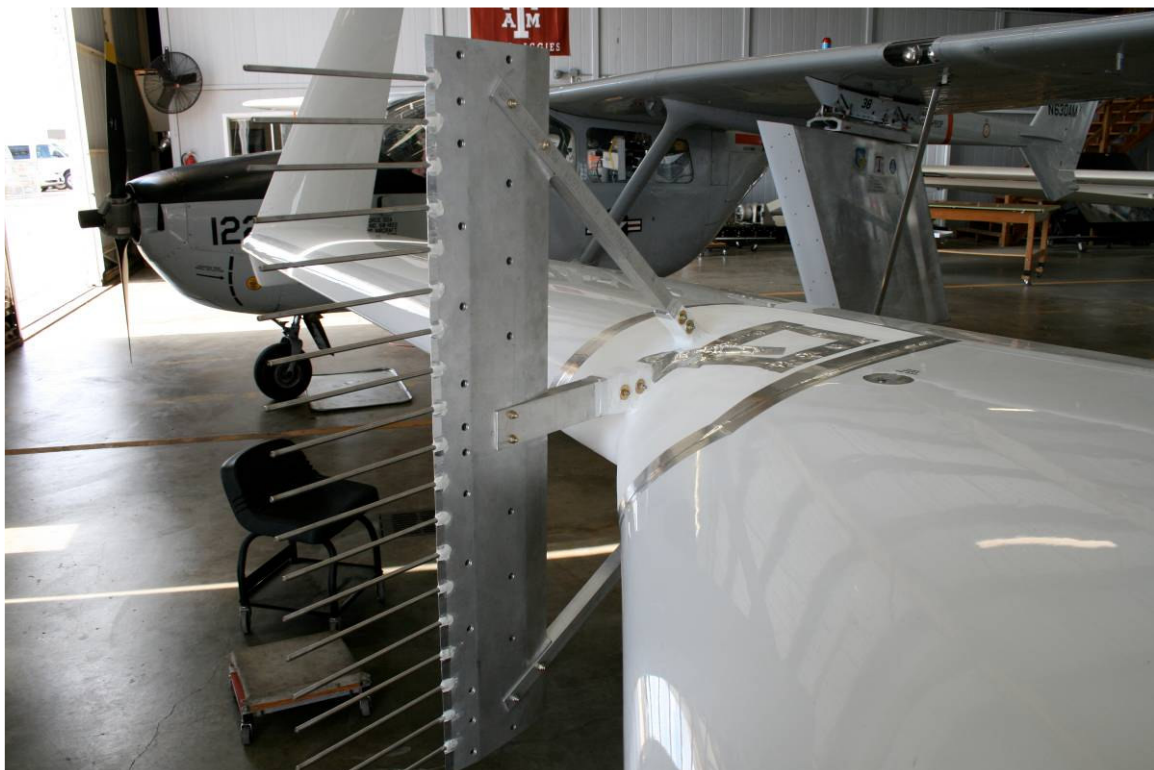
Figure A.103 Wing Glove and Pressure Rake Completed and Ready for Flight
