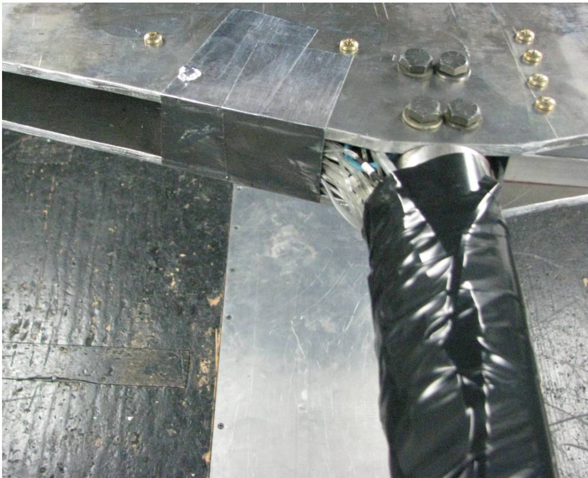
Figure A.133 Mounting of Pressure Rake to the Sting with Pressure Lines and Data Cables Secured in the Wind Tunnel
