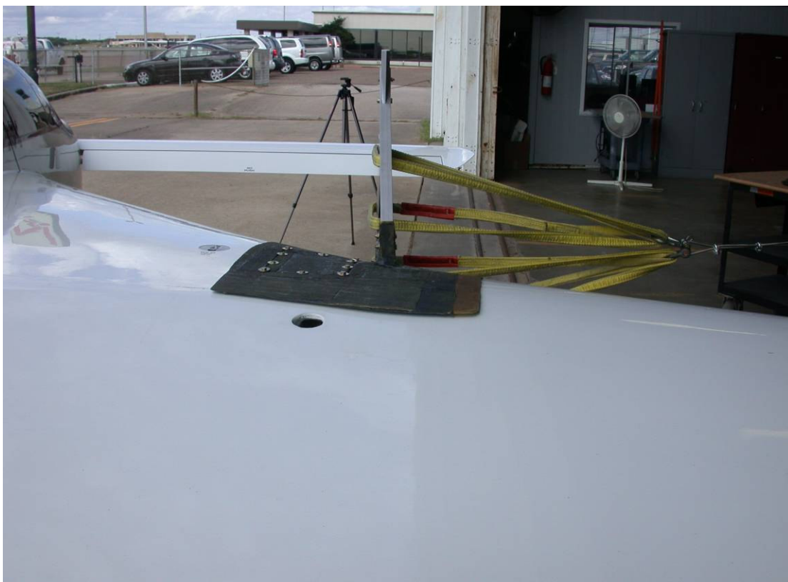
Figure A.100 Side Load of 86 kg Applied to the Pressure Rake While Mounted to the Aircraft
