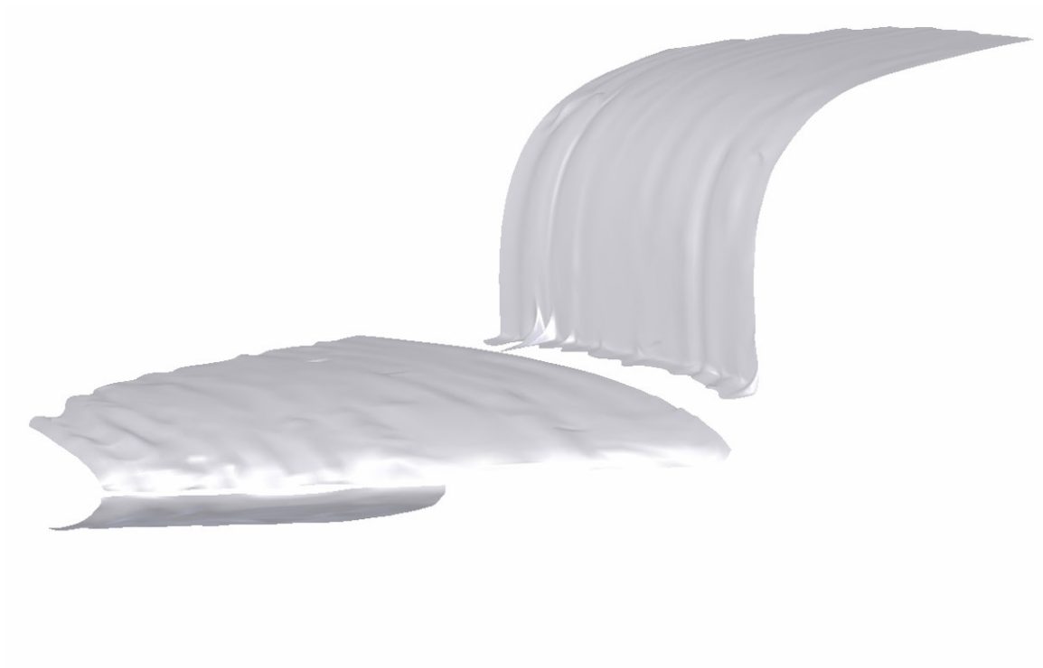
Figure A.11 Example of Rough Surface during Initial Lofting of Aircraft Surfaces
