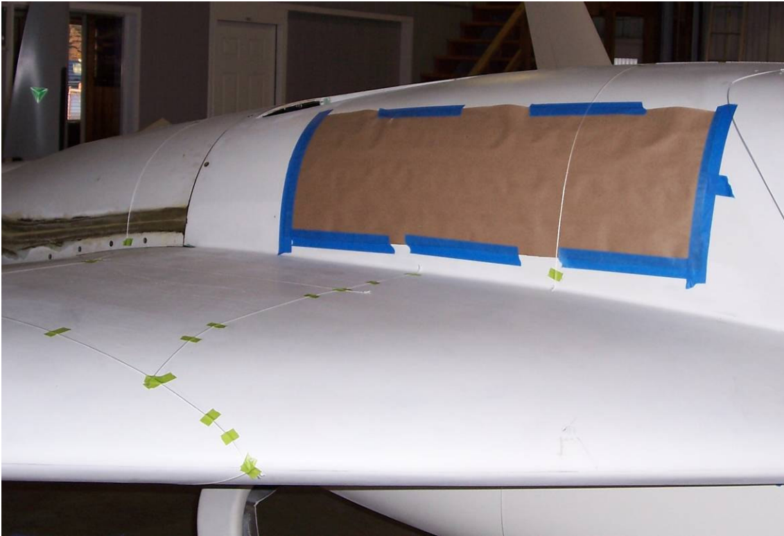
Figure A.7 Aircraft Split into 19 Sections for Measurements
