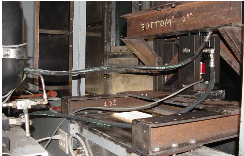
Figure 59: Structure to support the actuator and transfer the load
