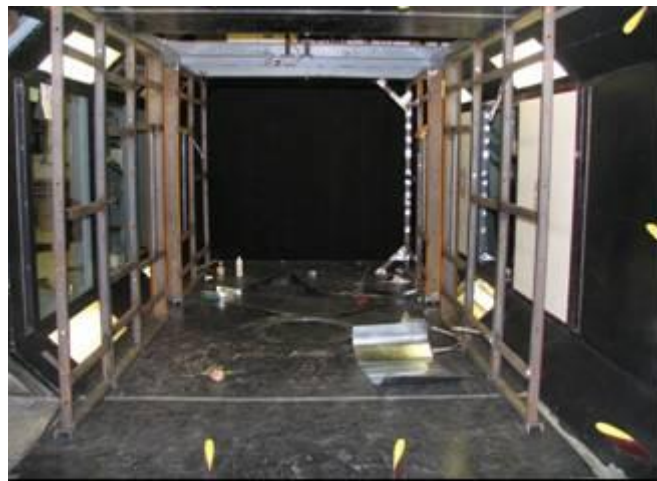
Figure 38: Left and right wall of the test section with frames
