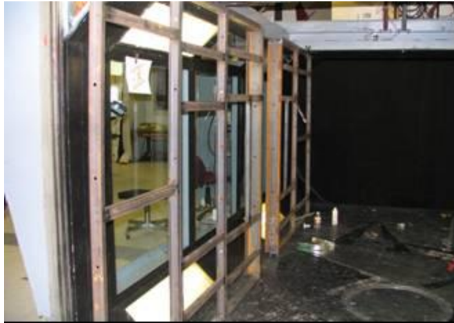
Figure 37: Left wall of the test section with frames
