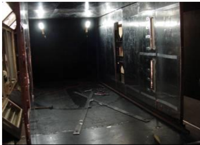
Figure 39: Right wall of the test section with aluminum sheet
