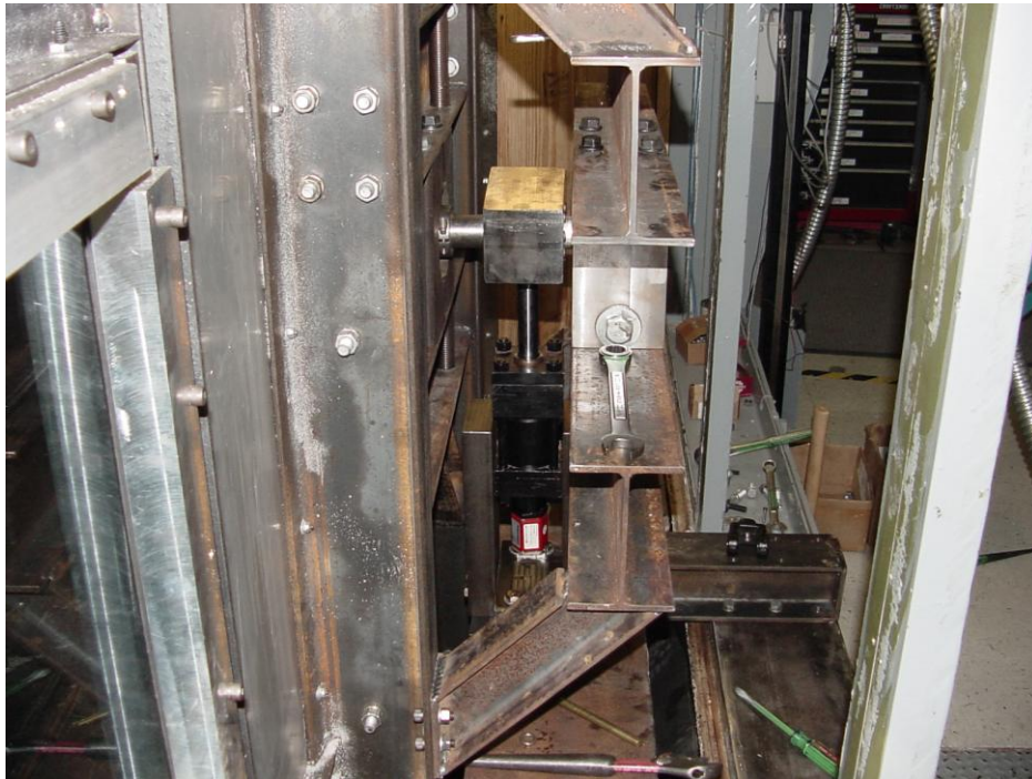
Figure B-11 Close up view of the wing with actuator and support structure
