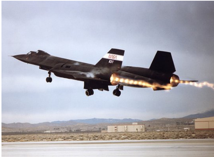
Figure 2. Mach disk ignition from the afterburner of a Lockheed-Martin SR-71 Blackbird 6 .
