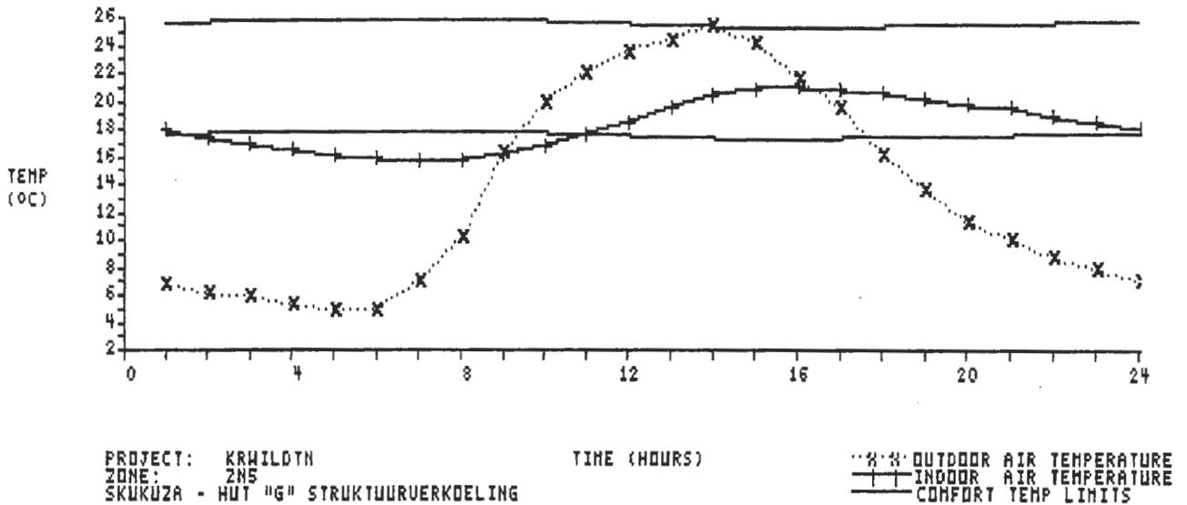
Figure 6. Structural night air cooling with cavity wall for winter conditions
