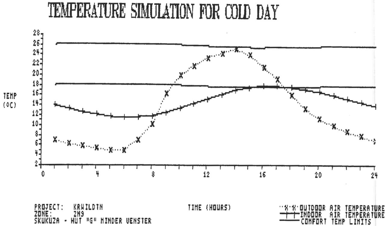
Figure 8. Elimination of west window for winter conditions
