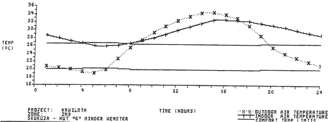
Figure 7. Elimination of west window for summer conditions
