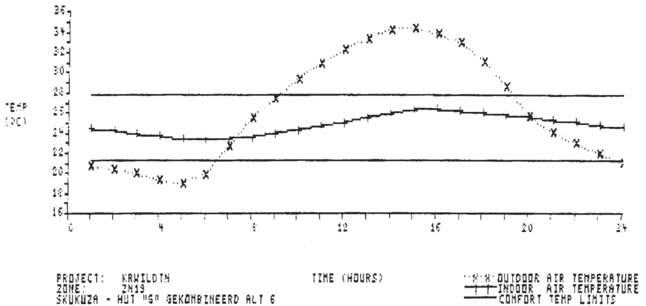
Figure 11. Underground air pipe, ceiling fan for summer conditions
