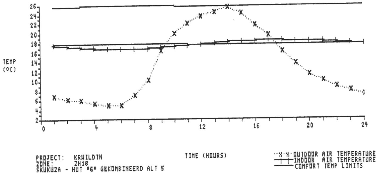
Figure 10. Cavity filled with 50mm polystyrene plus 80% direct evaporative cooling for winter conditions
