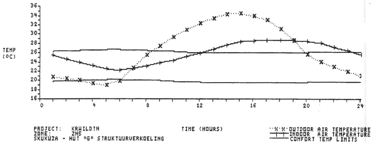
Figure 5. Structural night air cooling with cavity wall for summer condition
