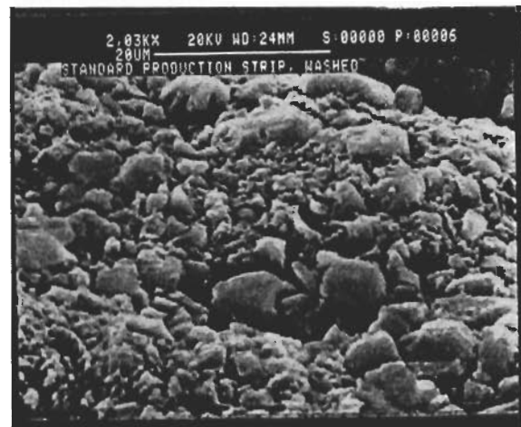
Figure 6. Desiccant Surface After Washing
