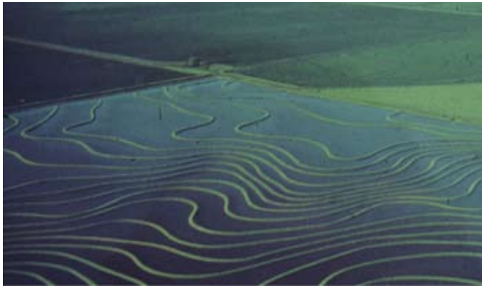
Aerial view of rice fields. Above: Contour graded, with closely spaced and curving levees. Below: Bench graded, with fewer levees that are straight and further apart.
