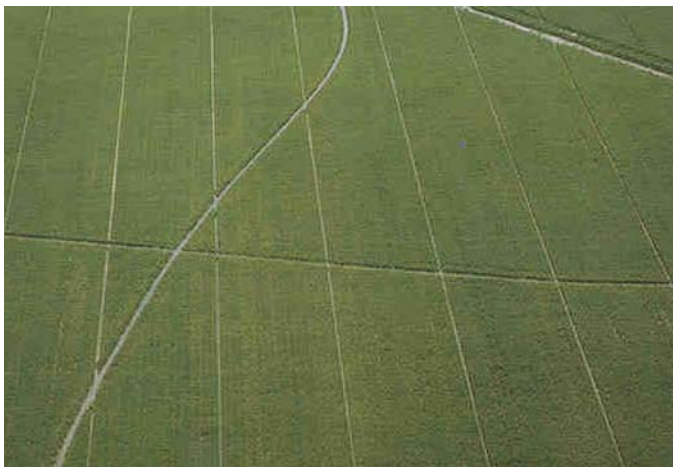
Aerial view of rice fields. Above: Contour graded, with closely spaced and curving levees. Below: Bench graded, with fewer levees that are straight and further apart.
