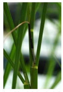
Pictured above is the hypodermic-like thermocouple that measures the internal temperature of the rice plant.
