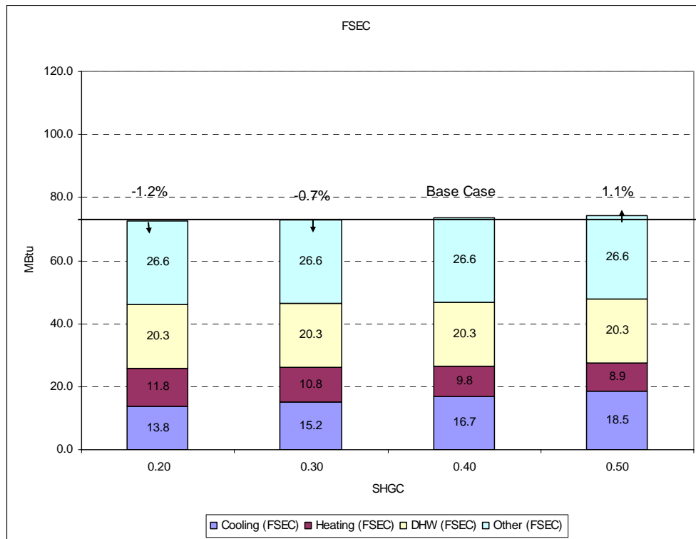
Figure 38. SHGC (FSEC) without the duct leakage.
