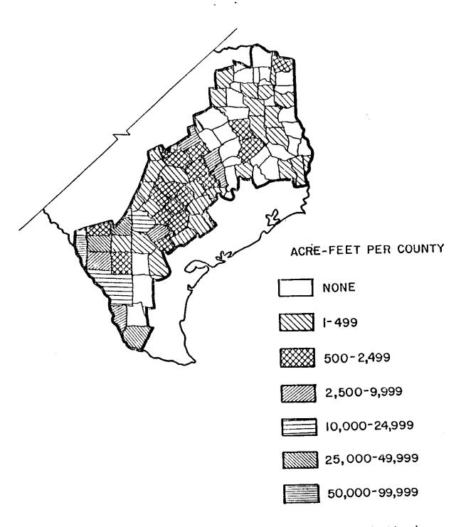
Figure 31. Average acre-feet of surface water used for irrigation by county in the Texas lignite belt.
