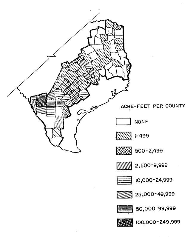
Figure 32. Average acre-feet of groundwater used for irrigation by county in the Texas lignite belt.
