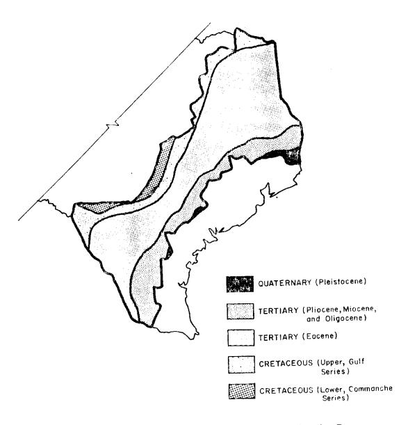
Figure 7. Principal surface geologic formations in the Texas lignite belt.
