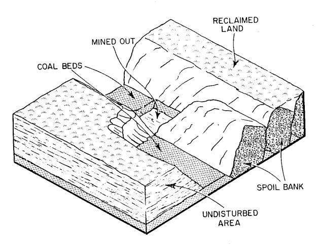
Figure 4. Schematic block diagram of lignite strip mining and reclamation.
