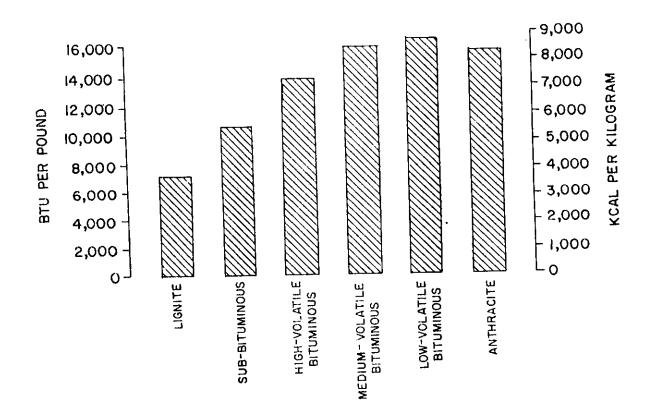
Figure 2. Heat content of various ranks of coal.
