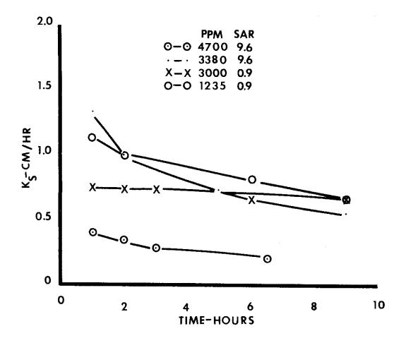
Figure 4. Saturated hydraulic conductivities (K ) in cm/hr as a function of time of cores of Clairemont silt loam (Reach 8) to distilled water after being leached with waters of indicated qualities for several hours.
