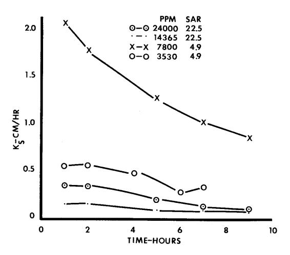
Figure 7. Saturated hydraulic conductivities (K<sub>)</sub> in cm/hr as a function of time of Yahola fine sandy loam and <sup>S</sup>Tipton silt loam (Reach 7) to distilled water after being leached with waters of indicated qualities for several hours.
