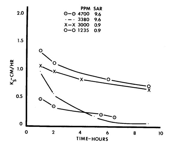
Figure 5. Saturated hydraulic conductivities (K<sub>s</sub>) in cm/hr as a function of time of Yahola fine sandy loam (Reach 13) to distilled water afterbeing leached with waters of indicated qualities for several hours.
