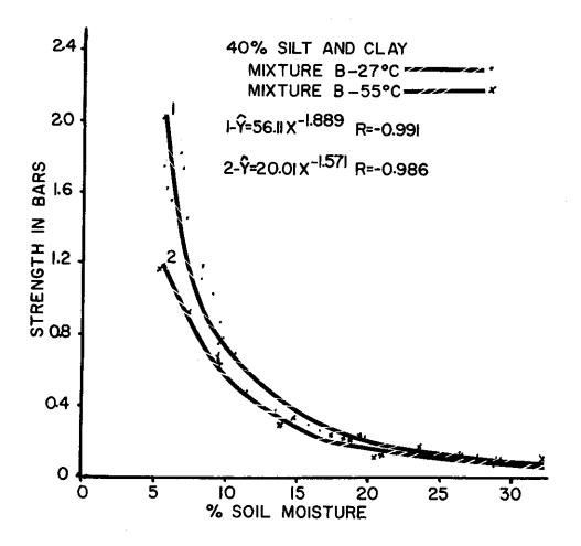
Figure 19. Relationship between percent of soil moisture and strength of briquets containing different amounts of silt-clay (Mixture B) and sand. Percent of sand is 40%.
