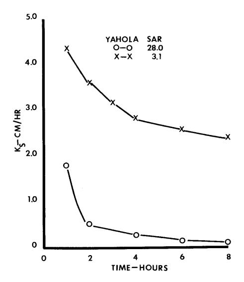
Figure 9. Saturated hydraulic conductivities in cm/hr as a function of time of Spur silt loam (Reach 14) to distilled water after being leached with water of indicated qualities for several hours.
