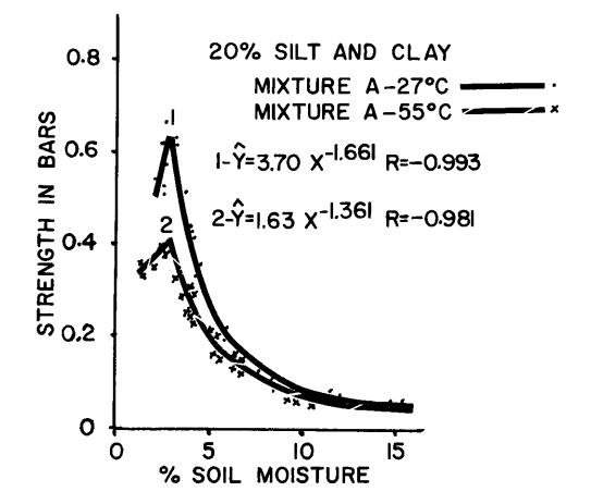
Figure 15. Relationship between percent soil moisture and strength of briquets containing different amounts of silt-clay (Mixture A) and sand. Percent of sand is 60%.
