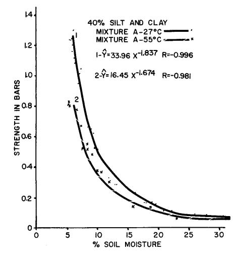
Figure 16. Relationship between percent soil moisture and strength of briquets containing different amounts of silt-clay (Mixture A) and sand. Percent of sand is 40%.
