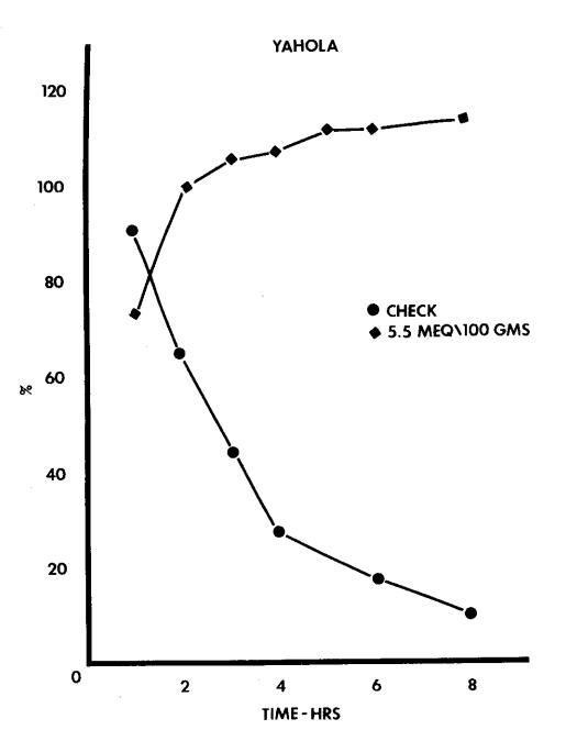
Figure 13. The relative change with time in saturated hydraulic conductivity (K ) to distilled water of the 0-3 inch depth of a <sup>S</sup>Clairemont silt loam in Reach 8 not treated and surface treated with ll meq/100 gms of concentrated  $H_2SO_4$ .
