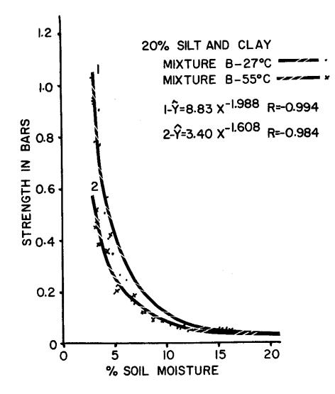
Figure 18. Relationship between percent soil moisture and strength of briquets containing different amounts of silt-clay (Mixture B) and sand. Percent of sand is 60%.
