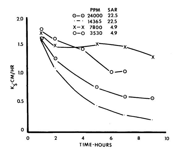
Figure 6. Saturated hydraulic conductivities (K ) in cm/hr as a function of time of Tipton silt loam (Reach 13) to distilled water after being leached with waters of indicated qualities for several hours.
