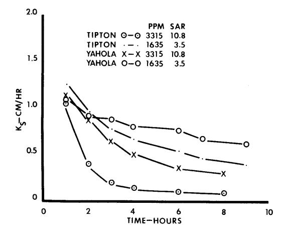
Figure 8. Saturated hydraulic conductivities in cm/hr as a function of time of Yahola fine sandy loam (Reach 14) to distilled water after being leached with water of indicated qualities for several hours.
