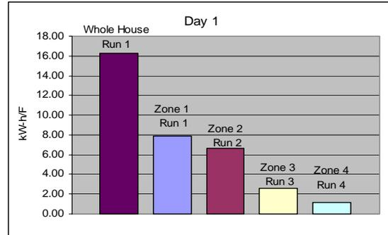
Figure 9: Day 1 comparison of furnace and fan energy required to heat zones 1-4 to the energy required to heat the whole house.
