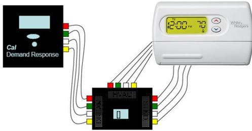
Figure 3: Wireless HVAC actuator and thermostat interface.
