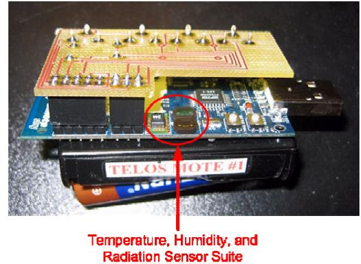
Figure 1: Tmote with full sensor suite: temperature, humidity, photosynthetically active radiation, and total solar radiation.
