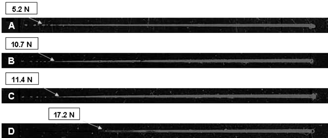
FIG 15. Processed images of Systems A-D showing onsets of visible damage obtained using the grayscale threshold option in ImageJ and corresponding critical loads.
