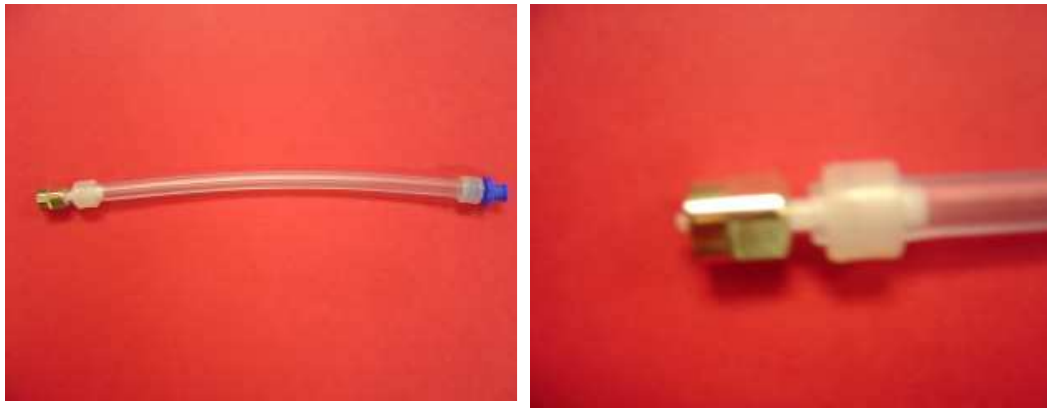
Fig. D-3 and D-4. The new auxiliary water port fitting after the pressure test.
