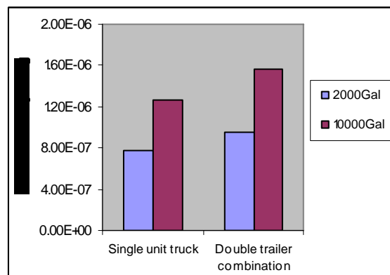
Figure 3.14. Effects of container capacity and truck configuration on the incident frequency.
