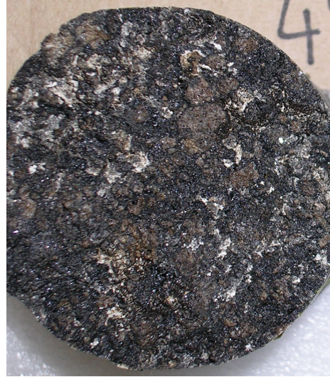
Figure 5.6. Failure Plane of Moisture Conditioned Sample After Dynamic Creep Test.
