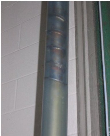
Figure 7.20 The Auger Tool in the downhole string (6 th floor)
