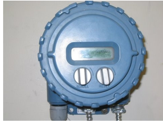
Figure 7.17 Air flow and temperature recorder Elite Type (sensor model CMF050) reading from Coriolis meter
