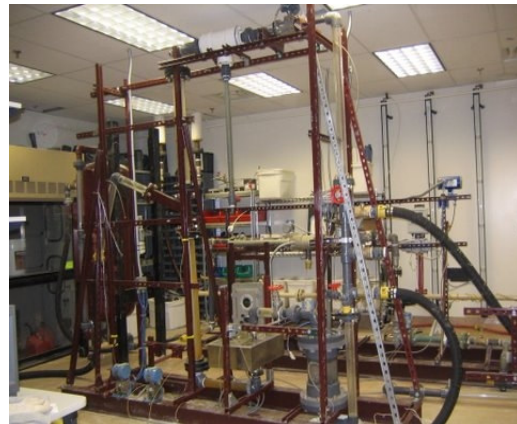
Figure 7.23 Setup of the cyclone separator and the buffer vessel
