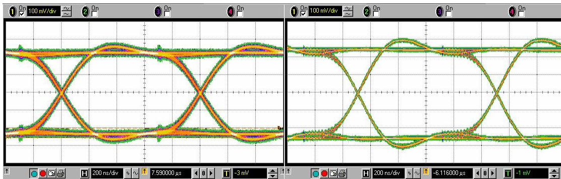
Figure 53: Uncompensated and Compensated PHY Eye at 2 Mb/sec
